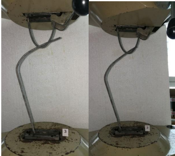
Fig. 6 Progress of the tensile test of wire – unfolding the bend. (Sample no.3 in two different stages)
