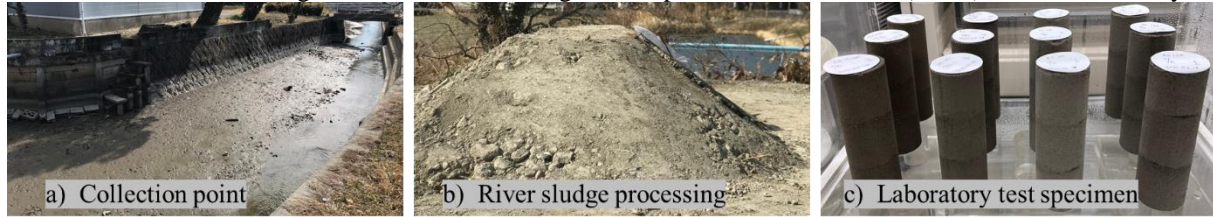
Fig. 1 (a) Location of river sludge collection, (b) River sludge processing on-site, (c) River sludge test specimen.
