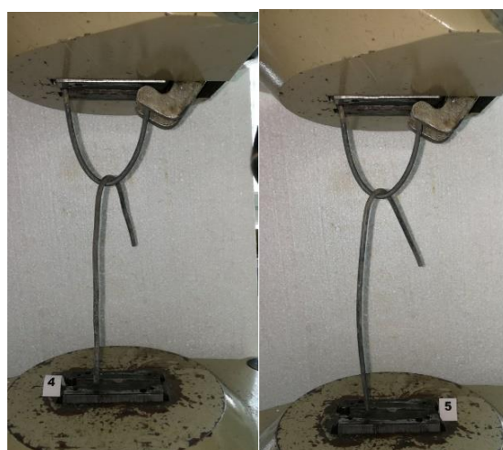
Fig. 5 Progress of the tensile test of wire – unfolding the bend. (Sample no. 4 at the start of the test – left, sample no.5 during the test)
