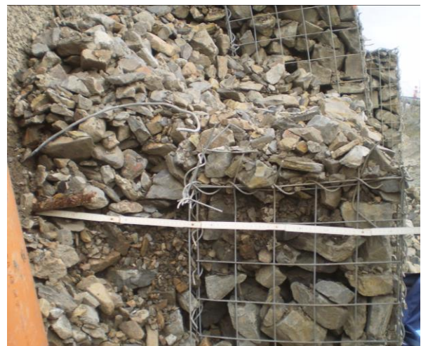
Fig. 3 Detail of steel wire attachment after reaching its bearing capacity
