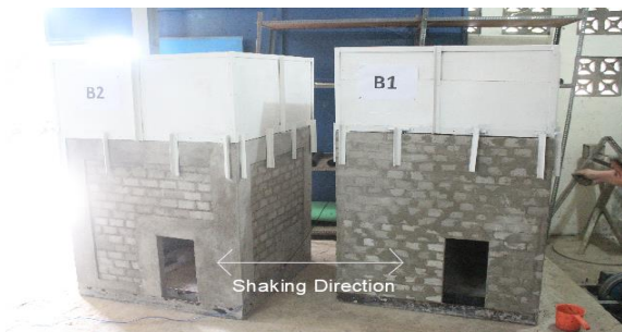
Fig. 9 Specimens that have been tested with 0.3g input motion and no applied additional load.
