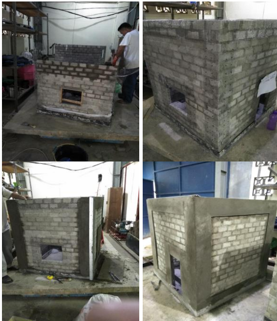
Fig. 6 Construction process of B2 specimens.
