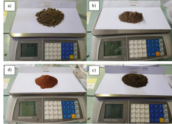
Fig. 3 Equivalent weighing of test sediment samples a) Ex. Field Sediments, b) Passed sieve #400 Ex. Stone Crusher, c) Passed sieve #400 Ex. Coal, and d) passed sieve #400 Ex. Brick in the Fluid Laboratory ITB (2022)
