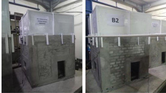
Fig. 11 Specimens that have been tested with an input motion of 1g and an additional uniform load of 500 kg.
