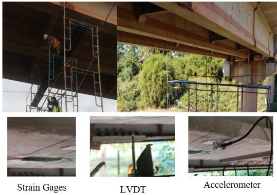
Fig. 9 Installation testing instruments for Brg. No.5
