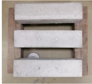
Fig. 3 The specimen after contact tips were attached
