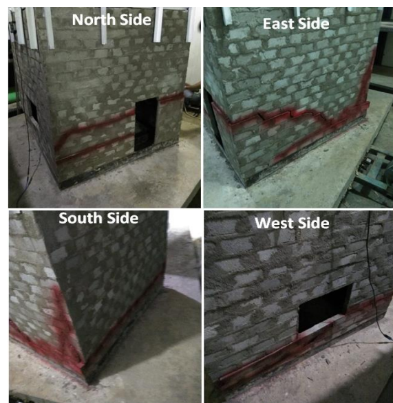
Fig. 10. Specimens that have been tested with Input motion of 0.6 g and an additional uniform load of 200 kg.
