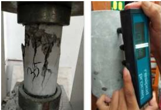
Fig. 3 Compressive test and Chloride penetration test of concrete
