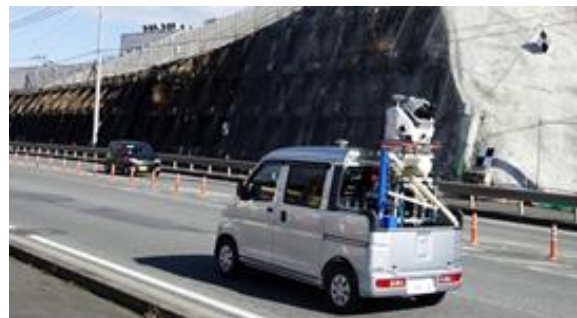
Fig.1 Photograph of slope observation using the MMS
