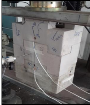
(a) Cracks on prism
