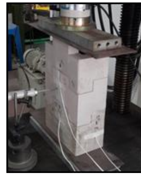
(b) Prism test set-up
