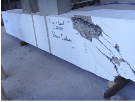
Fig. 10: 'B1-5' Shear Failure at the Load of 280 kN
