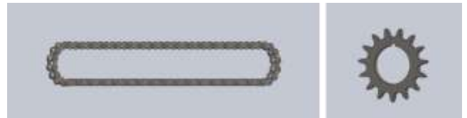
Figure.4: Chain and sprocket for dry land power weeder
