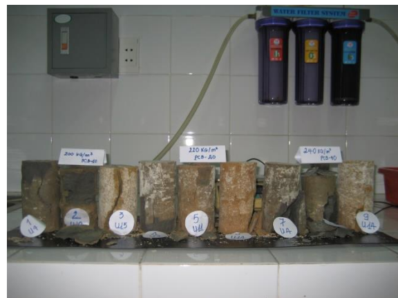
Fig. 9 Specimens sunk in salinity water after 2 years
