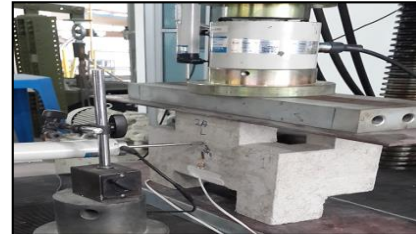
(a) Stretcher block test set-up
