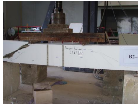
Fig. 17: Cracks Pattern of Beam 'B2-5
