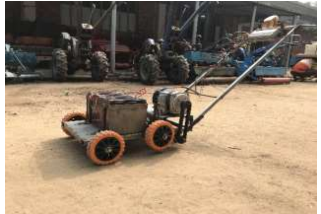
Figure.7: Pictorial view of Battery operated dry land rotary weeder
