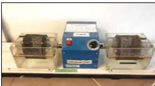
Fig. 7 Slake Durability Equipment
