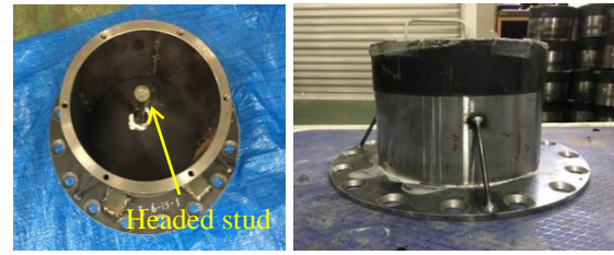
Fig. 3 General view of specimen before casting concrete.
