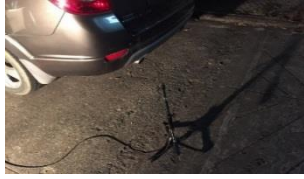
Fig. 7 A position of the microphone : a position at the rear of the exhaust pipe with a 45-degree angle to that pipe and a 0.5-meter far distance
