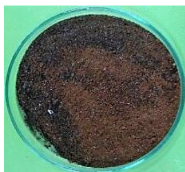
Fig. 3 Crude extract of tannin extracted with 95% ethanol, 80°C at 1:10 g.mL -1 proportion
