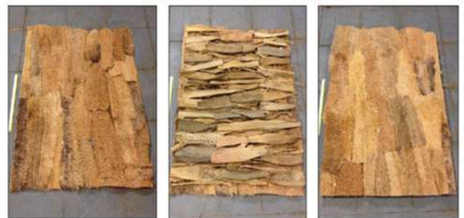
Fig. 2 Three layers of geotextile
