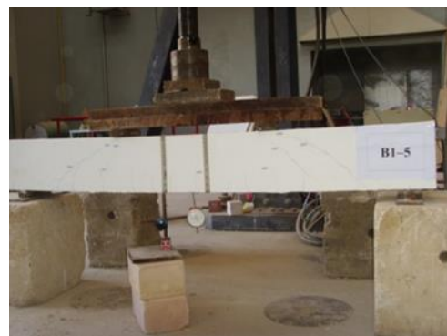
Fig. 9: 'B1-5 Cracks at the Load of 100 kN
