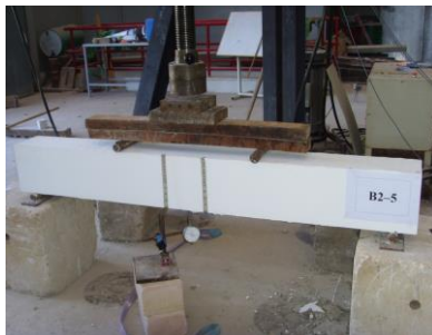
Fig.18: Distribution of Strain Gages
