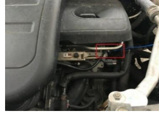
Fig. 2 A position of the vibration sensor : the surface of the engine pistons
