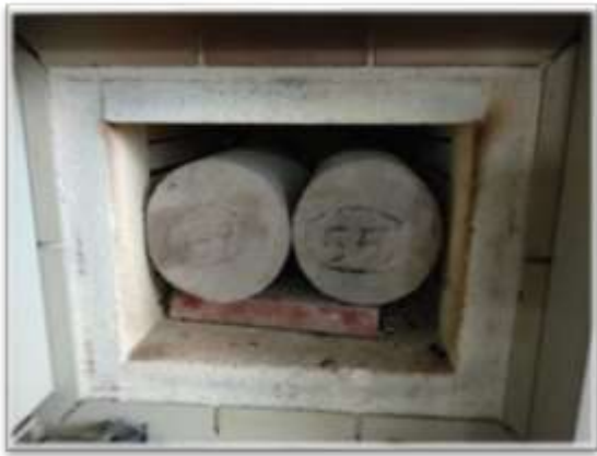
Fig. 4 High temperature exposure in oven
