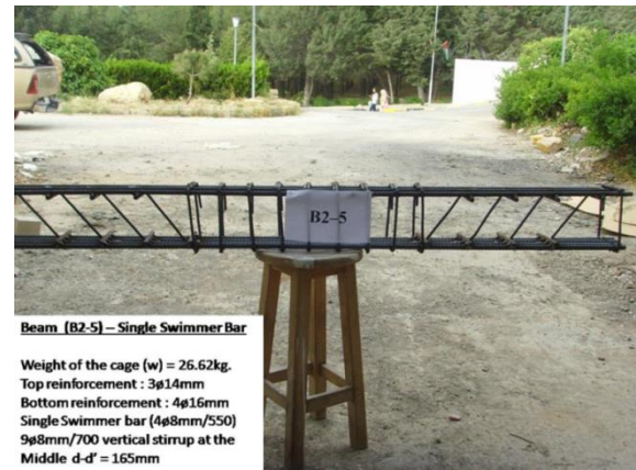
Fig. 4: Steel Cage Reinforcement of Beam 'B2-5
