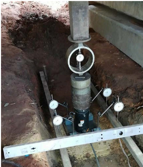
Fig. 6 The installation of plate bearing test in the wet pit
