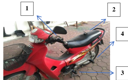
Fig. 3 Experimental allocation of accelerometers over the specimen motorcycle; (1) left hand, (2) seat, (3) left front footrest, and (4) left rear footrest.
