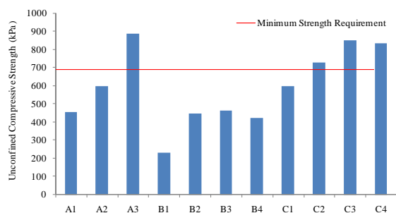
Fig. 9 Unconfined compressive strength of soil mixed with an admixture for each mixture in 7 days curing time
