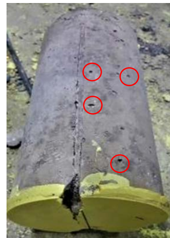
Fig. 4 Identified porous on the concrete surfaces.
