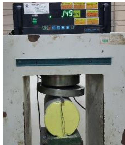
Fig. 8 Tensile strength of FRC with various fiber interlocking
