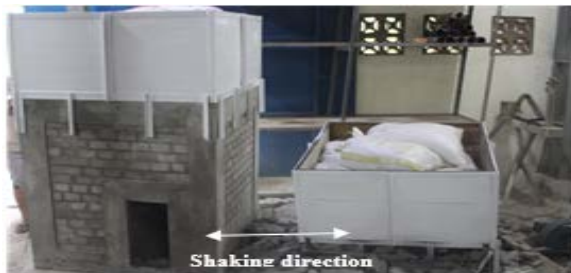
Fig. 15 The specimens with 500 kg additional uniform loads and 0.6g input motions (P5) at front side after testing.
