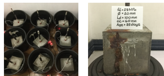
Fig. 1 Concrete cubes under accelerated corrosion
