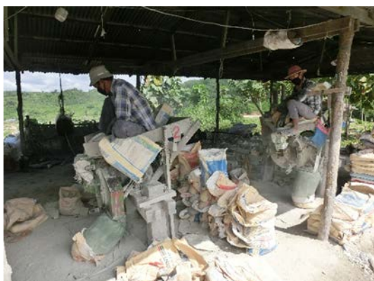
Fig. 3 Machine that powders gold ore
