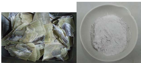
Fig. 1 Waste Pen Shells Before and After Calcination
