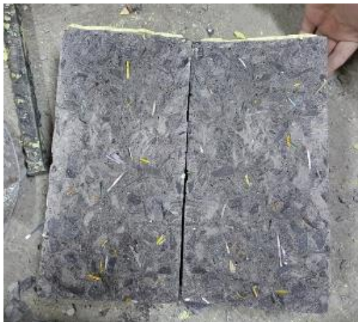
Fig. 10 Fiber sticking out of concrete surfaces.
