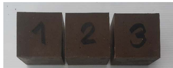
Figure 3. The sample of fluidized bed coal-bark fly ash geopolymer mortar containing additives
