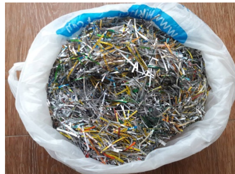
Fig. 2 Sample of fiber with width of 2mm and length 40mm without interlocking shape.
