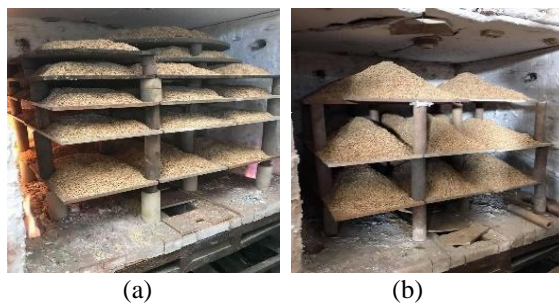
Fig. 1 Layering of RH on slab plates in two manners: (a) thinly flat (b) triangular prism
