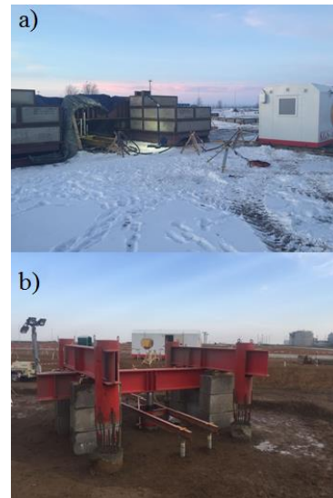
Fig. 6 Field pile test by SCPLT method a) platform b) anchors pile.
