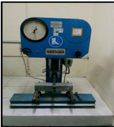
Fig. 6 Flexural test on beam specimen
