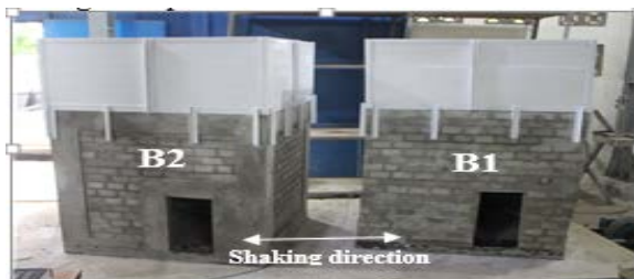
Fig. 8 The specimens without additional uniform loads (P1) after testing
