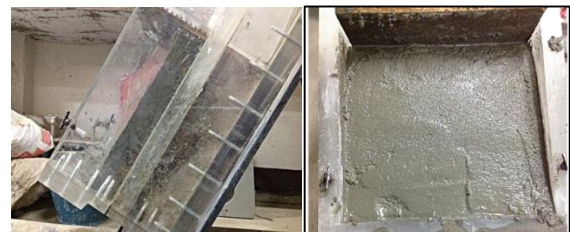
Fig. 4 Sagging and Build-up thickness of mortar.
