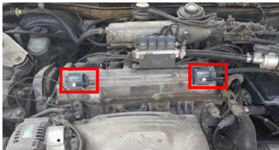
Fig. 1 Sensor allocation design : the first stage
