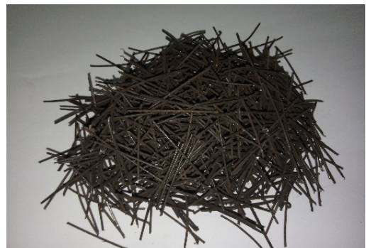
Fig. 3 The 4cm length of steel fiber extracted from waste tyre
