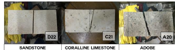
Fig. 7 Failure of masonry blocks due to flexure
