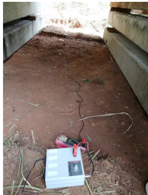
Fig. 4 Measurement matric suction by using KU tensiometer
