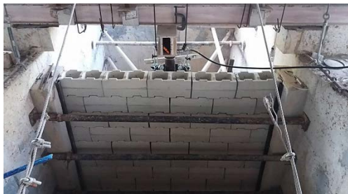
Fig.9 Half nano block test set up (Front view)
