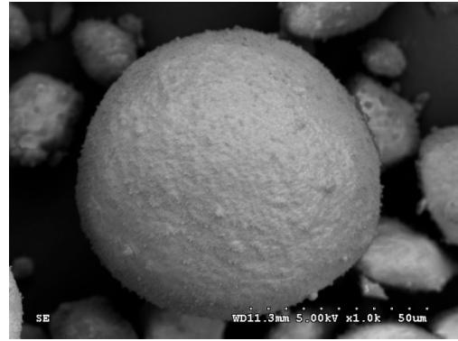
Fig.5 SEM photograph of silica fume
