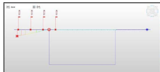
Fig. 13: Location of wheels load on the deck generated by MIDAS Civil software
