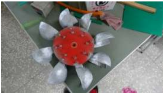
Fig. 13 Turbine blade after assembly
