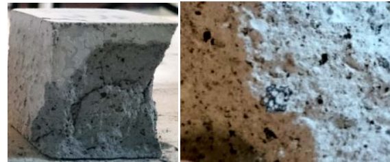
Fig. 5 The failure plane of shotcrete mortar used bottom ash as fine aggregate.
