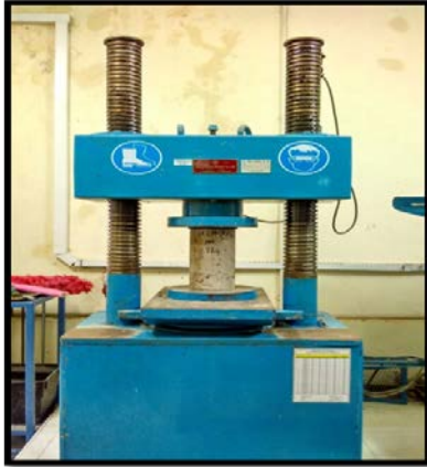
Fig. 4 Compressive test on cylindrical specimen
