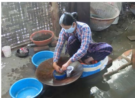
Fig. 4 Squeezing the gold-mercury amalgam
