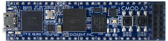
Fig. 2 Platform of cmod A7-35T breadboardable artix-7 FPGA module.
