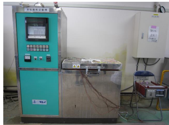
Fig.7 Freeze and thaw test machine
