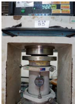
Fig. 1. Test model with compressive test machine
