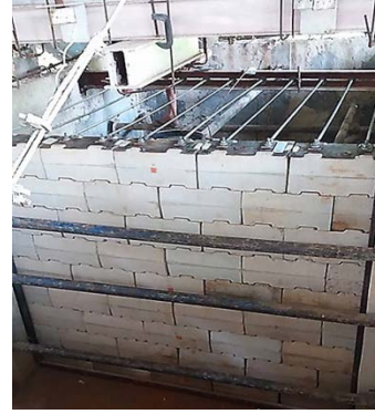
Fig.11 Half nano block test with reinforced bar anchorage (Front view)
