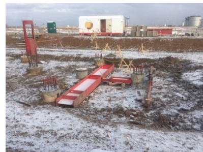
Fig. 10 Static Lateral Pile Loading Test.
