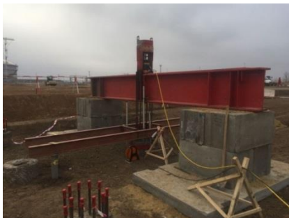
Fig. 8 Static Tension Pile Loading Test.
