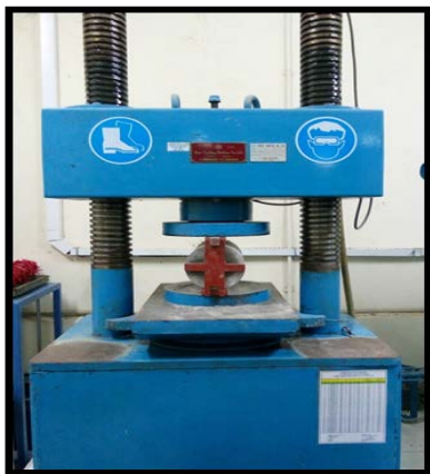
Fig. 5 Splitting tensile test on cylindrical specimen
