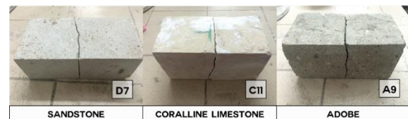
Fig. 4 Failure of masonry blocks due to shear
