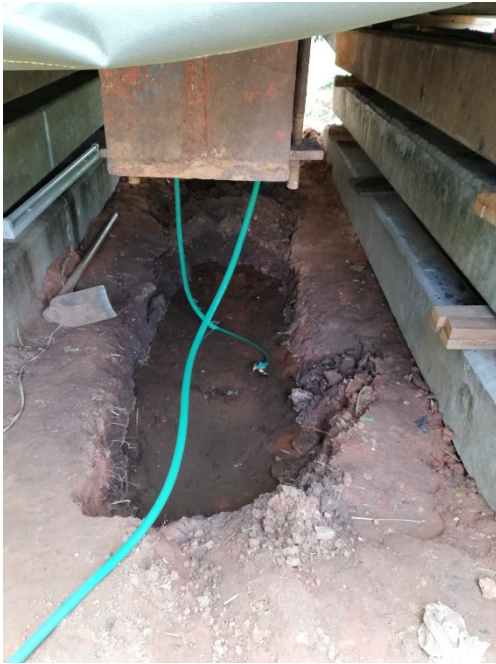
Fig. 5 Wetting pit (soaking for 4 days)
