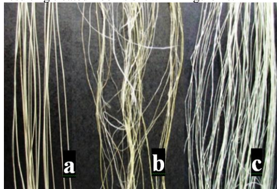
Figure 1 (a) raw abaca fiber, (b) alkali pretreated abaca fiber and (c) alkali- \text{Al}_2(\text{SO}_4)_3 treated abaca fiber
