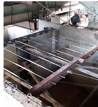
Fig.7 Half nano block with reinforced bar and anchorage test set up (Back view)
