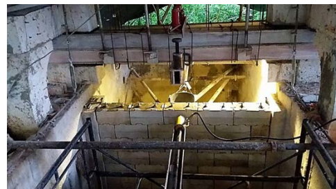
Fig.12 Composites elastic modulus test set up (Front view)
