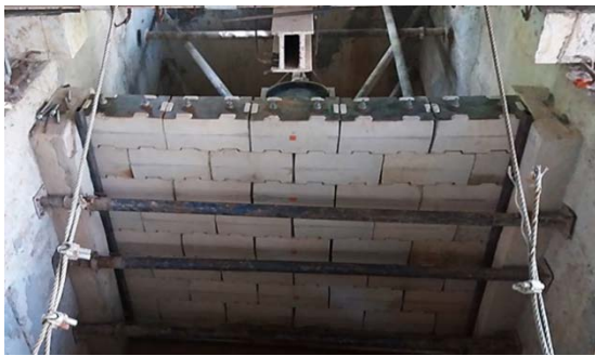
Fig.10 Half nano block test with reinforced bar (Front view)
