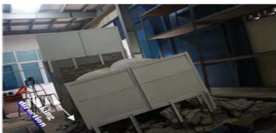
Fig. 16 The specimens with 500 kg additional uniform loads and 0.6g input motions (P5) at east side after testing.
