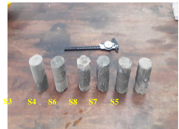
Fig. 2 Cracked samples joined with cement paste.
