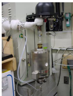
Fig. 3 Sample and reference quartz pans or crucibles utilized in the DTA measurements, remote view while the furnace is open (lowered).
