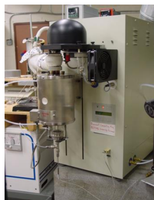
Fig.1 TG device consists of small furnace.
