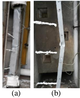
Fig. 7 (a) Test set-up (b) buckling of box-up column
