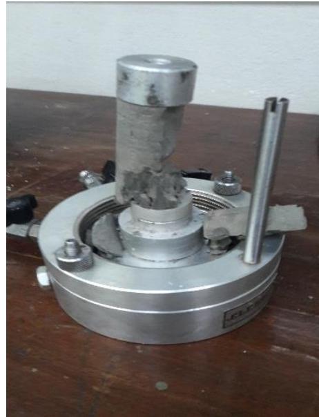
Fig.12 Typical failure of cement joined sample
