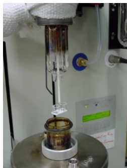
Fig. 2 Sample and reference quartz pans or crucibles utilized in the DTA measurements close view.
