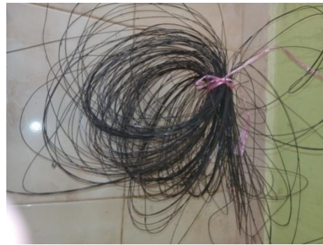
Fig. 2. Steel Fiber Extracted From Waste Tyre
