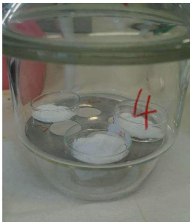
Fig. 6 Desiccation jar measurement of triplicate salt samples with humidity controlled by reference salts placed in base of jar
