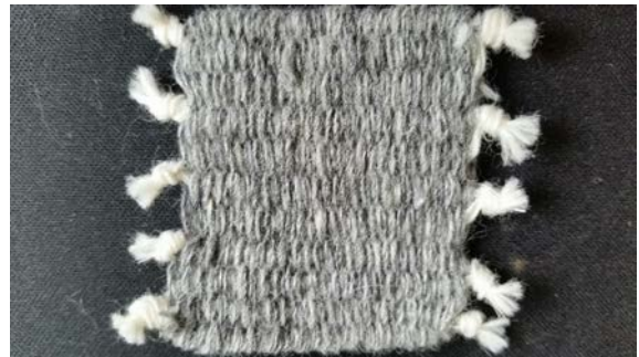
Fig. 5 Example of the proposed clad-removed POF based weave structure (plain weave)
