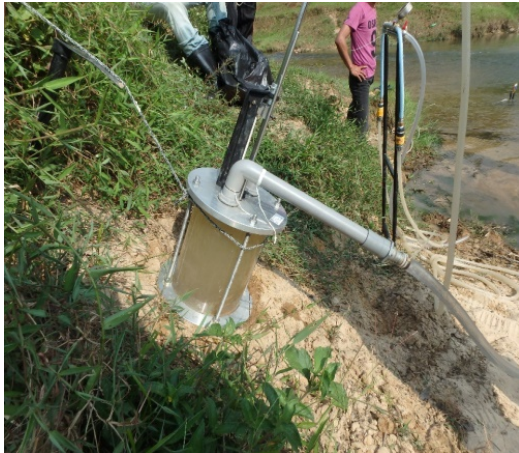
Fig. 1. JEd test at field location
