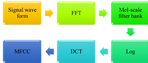
Fig. 1 The feature extraction process using MFCC.
