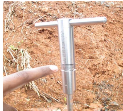
Fig.3 Filed vane shear test at site B
