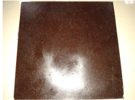
Fig. 1 Bio-composite board made from coco coir dust and LDPE pellets
