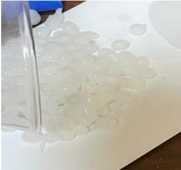
Fig. 1 Microcapsules made from Sunflower oil and calcium alginate.
