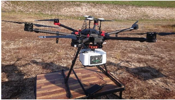
Fig. 1 Drone equipped with green laser scanner
