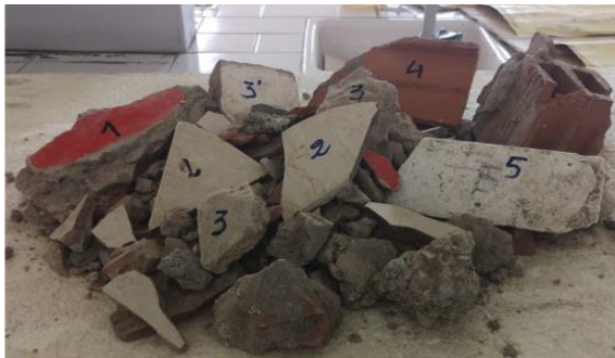
Fig. 1: representative samples of construction waste before crushing and grinding.
