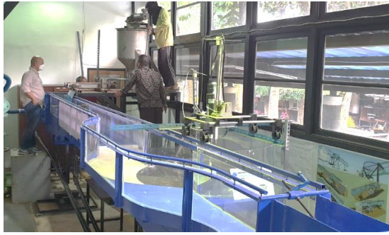
Fig. 6 Visual view of the undistorted physical model with a scale of 1:40
