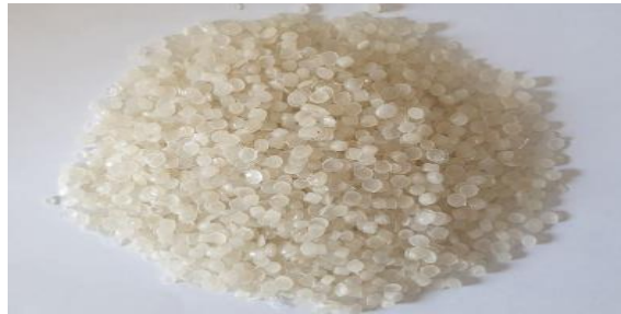
Fig. 4 Shape of plastic LDPE flattened round.
