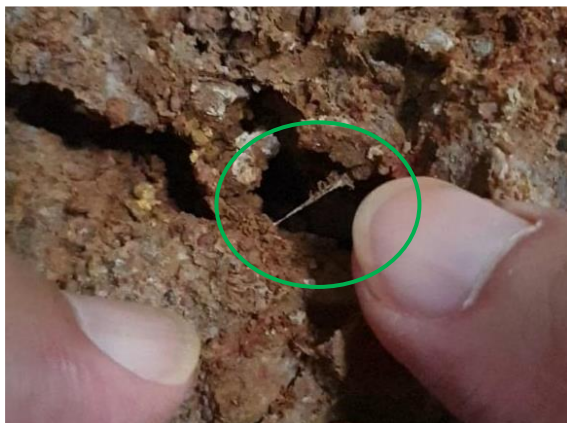
Fig. 5 Bond of Para-rubber of SCP.
