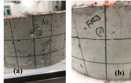
Fig. 11 Restrained shrinkage cracking (a) plain SCC (b) Fiber-Reinforced SCC.
