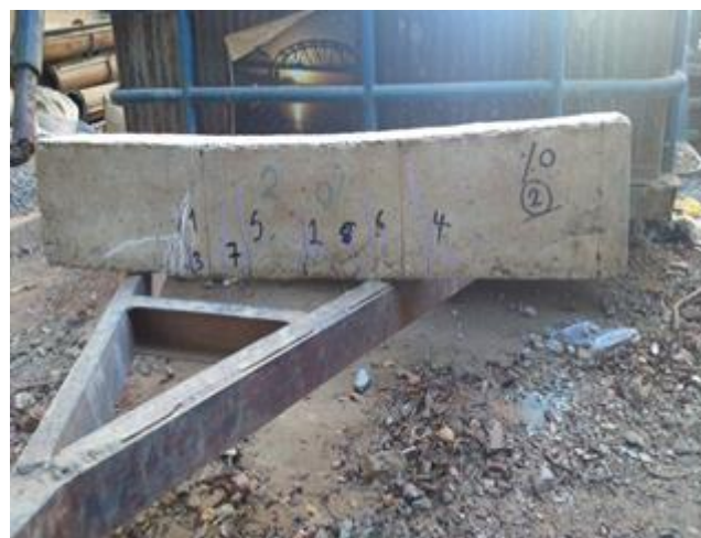
Fig. 8 Shear behavior of beam 0.0% fiber content
