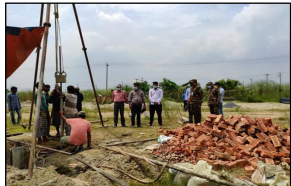
Fig. 2 Standard Penetration Test (SPT) setup
