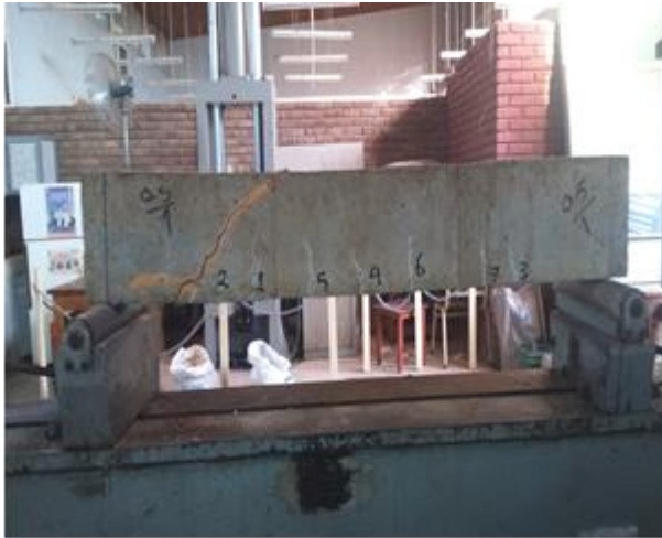
Fig. 11 Shear behavior of beam 0.0% fiber Content
