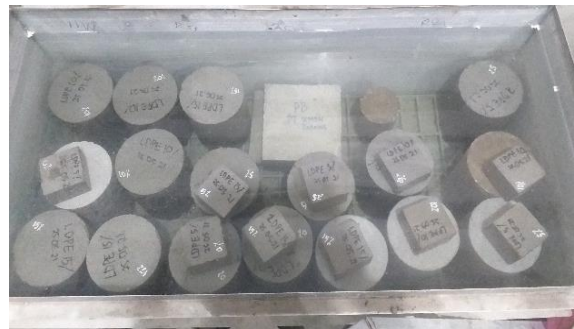
Fig. 6 The curing of test specimens.
