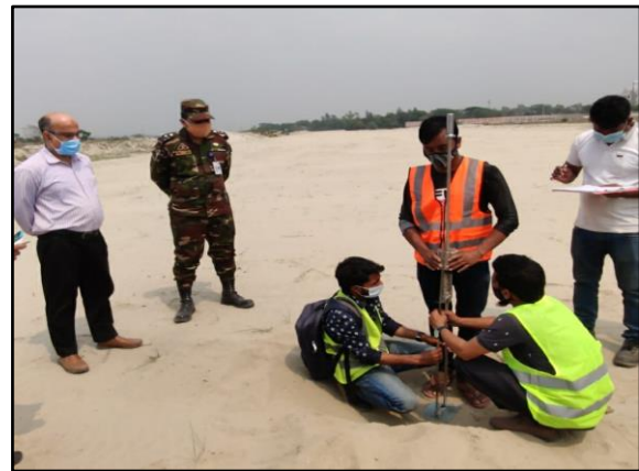
Fig. 6 Implementation of Dynamic Cone Penetration (DCP) test
