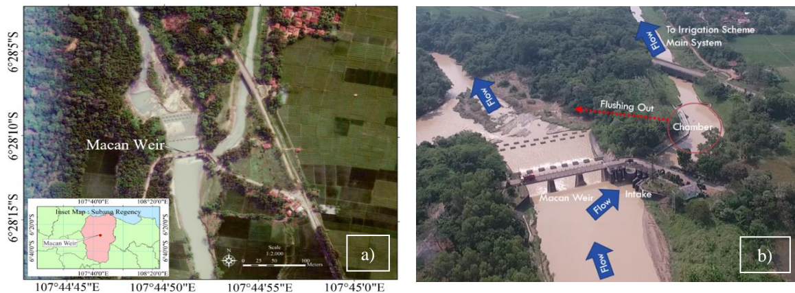
Fig. 2 a) Layout of Macan weir, 2 b) Propose of vortex desilting basins location at Macan weir
