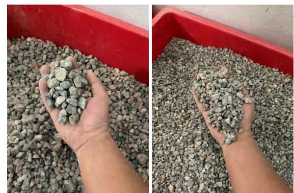
Fig. 3 RCA from CC of size 10-20mm (left), and 5-10mm (right)
