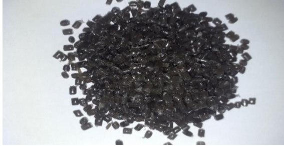
Fig. 3 Shape of plastic LDPE pellet.
