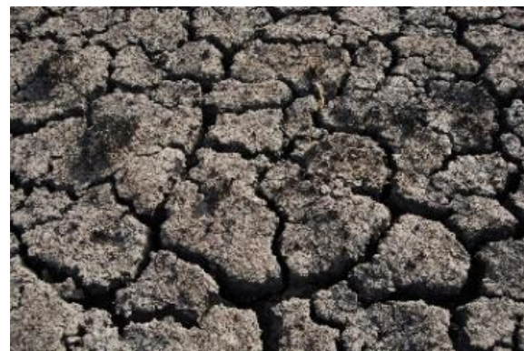
Fig. 2 Desiccation cracking in expansive natural soil (Source: http://geophilous.blogspot.com )
