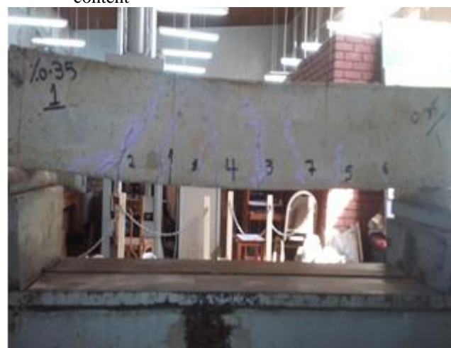
Fig. 10 Shear behavior of beam 0.35% fiber content
