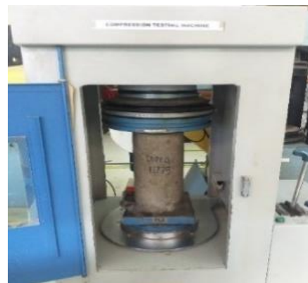
Fig. 7 Compressive strength test of cylinder test specimens.
