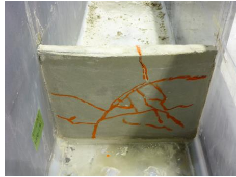
Fig. 13 Soil-cement cutoff wall after shaking.
