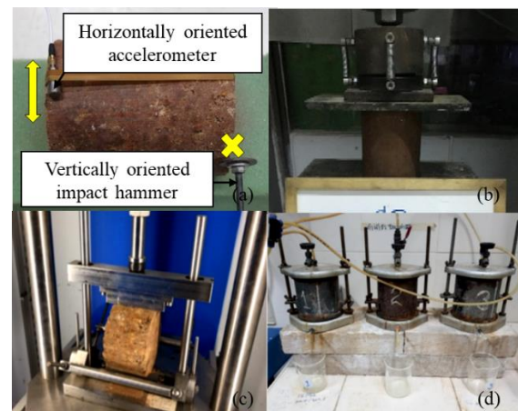
Fig. 2 Examples of (a) free-free resonance test (b) unconfined compressive strength test (c) indirect tensile strength, resilient modulus and fatigue resistance tests (d) soil permeability test
