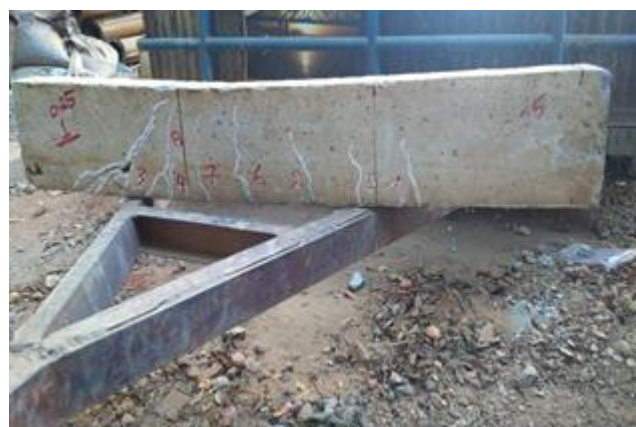
Fig. 9 Shear behavior of beam 0.25% fiber content
