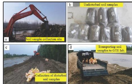
Fig. 4. Process of dredging, collection of undisturbed, disturbed soil samples
