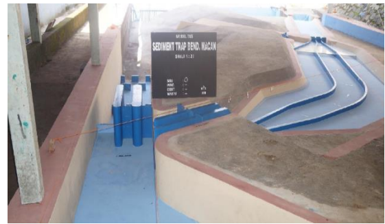
Fig. 7 Undistorted physical model test scaling 1:20 for conventional rectangular sediment trap
