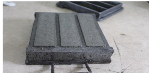
Fig. 3: Specimens of dimensions: 40×40×160 mm
