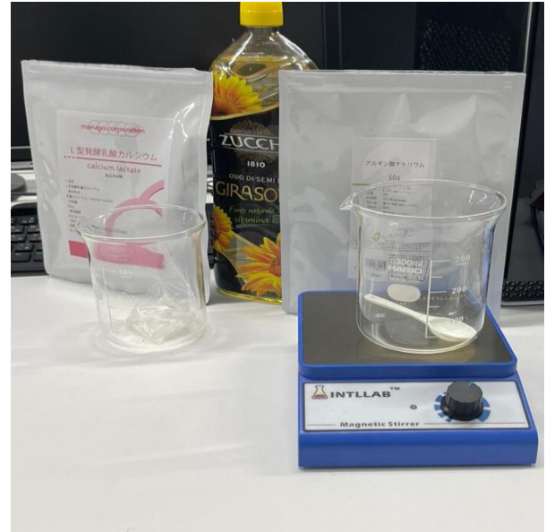
Fig. 2 Materials used to produce homemade capsules from sunflower oil.
