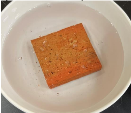
Fig.5 The generation of large and fine bubbles
