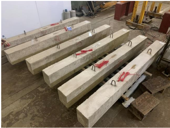
Fig. 7 Beams with installed sensors
