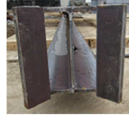
Fig. 2 Pile tip shape of soil-cement composite pile.
