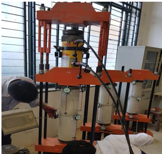
Fig. 5. Set-up of concrete creep measurements
