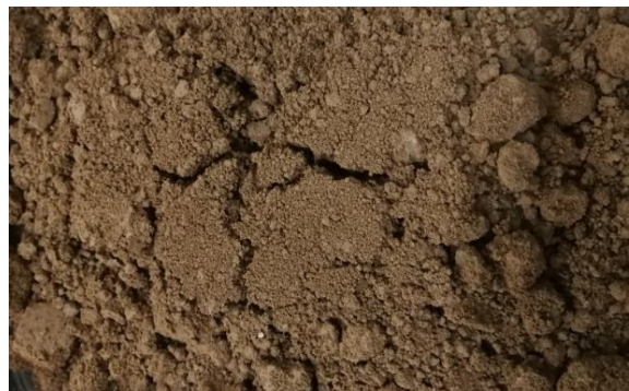
Fig. 2 Crack propagation in Kauswagan soil sample.
