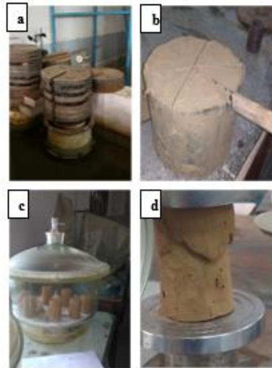
Fig. 1 a) Ko-Consolidation of soil b) reconstituted soil specimen c) soil sample kept inside desiccator, and d) Failure plane after testing.
