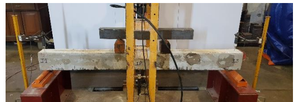
Fig. 4 Four-point bending test on a typical beam specimen
