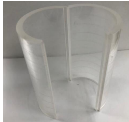
Fig. 6 Split mold for estimating self-standing height of RS specimens
