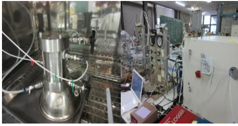
Photo. 2 Installed pore pressure sensors at steel mold, thermostat oven and burette for measurement of absorbed water.
