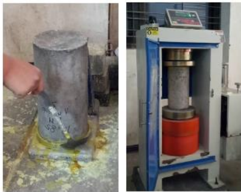
Fig. 4. Compressive test on cylindrical samples.
