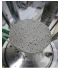
Photo. 3 Observed cracks on surface for unsaturated bentonite subjected to heating.
