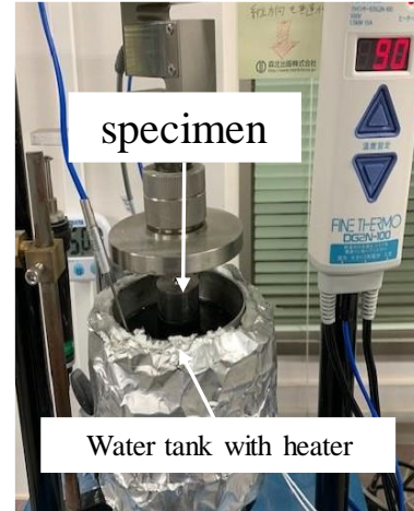
Fig. 4 Uniaxial compression test in a temperature environment
