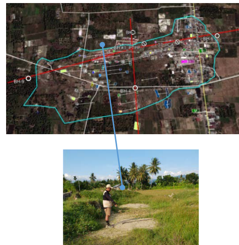
Fig. 5 One of sand boil at Lolu Village site
