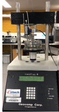
Fig. 3 Conventional oedometer apparatus used for the shear rate determination
