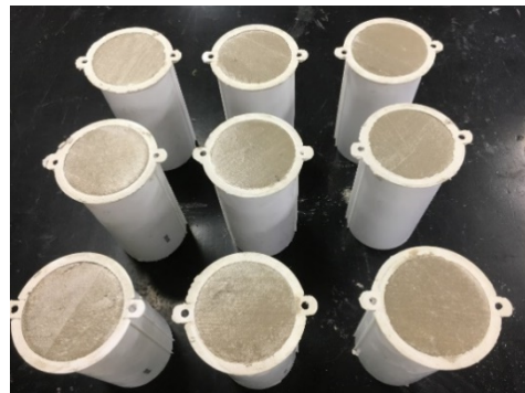
Fig.4 Cylindrical plastic mold ( \phi=100 mm, h=200 mm)
