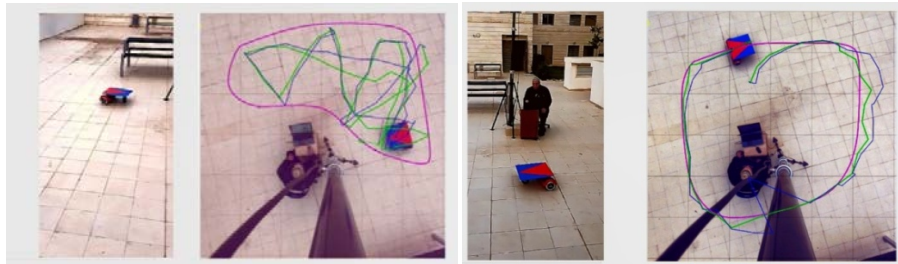
Fig 7. Two experimental tests - random movement in user predefined boundaries and user predefined route.
