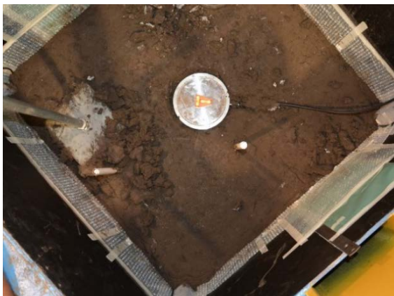
Fig.5 Installation of the soil pressure transducer
