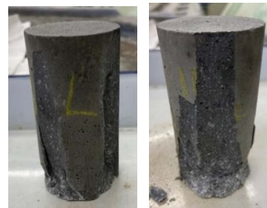
Fig.11 LPC-ME-MXS specimens after the 91-days-old compression test.
