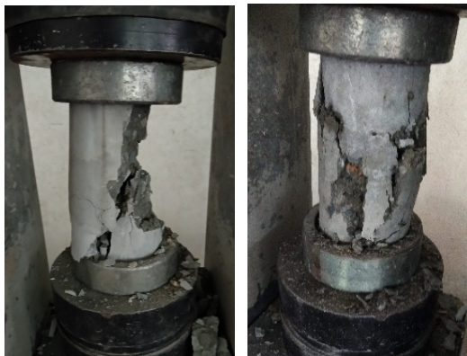
Fig. 5 Failure of concrete cylinder under compressive force.
