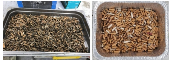
Fig. 5. CBs before encapsulation. Waste CBs (left) and oven dried and cleaned CBs (right).
