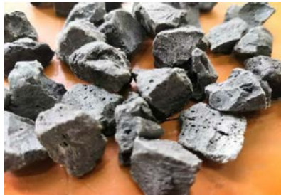
Fig. 2 Processed polypropylene (PP) aggregates
