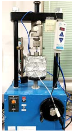
Fig. 2 Uniaxial compression tester
