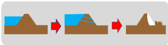
Fig. 3 Osmotic collapse process
