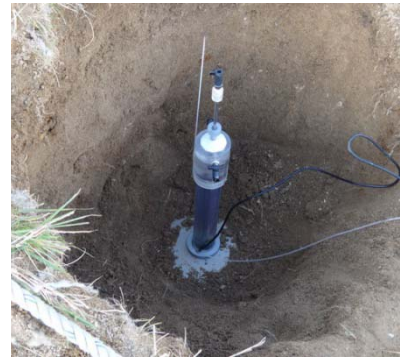
Fig. 9 Field water injection test.
