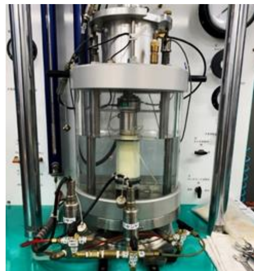
Fig. 4 Cyclic triaxial apparatus.
