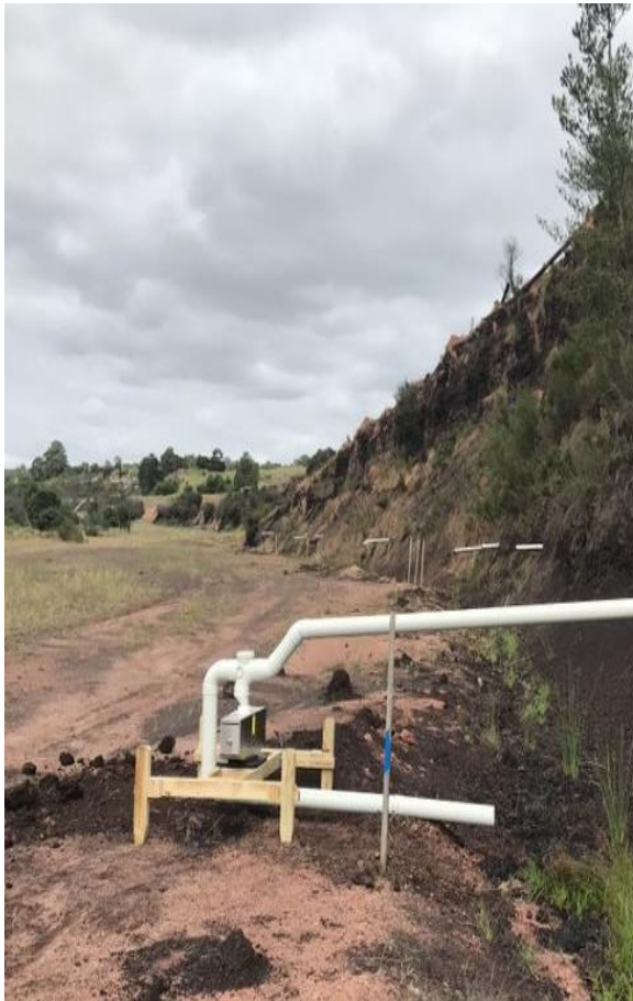
Figure 2: Flow meter connected to a selected bore
