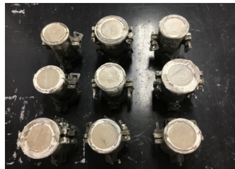
Fig.5 Steel cylinder formwork ( \phi=50 mm, h=100 mm)
