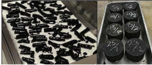
Fig. 2. Encapsulated CBs and a few dense asphalt samples used in the research conducted by Mohajerani et al. in 2017 [12].
