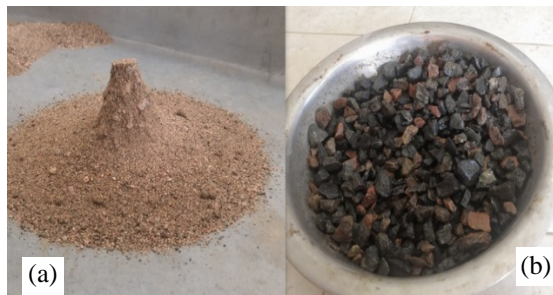
Fig. 1 Aggregate: (a) coarse, and (b) fine.
