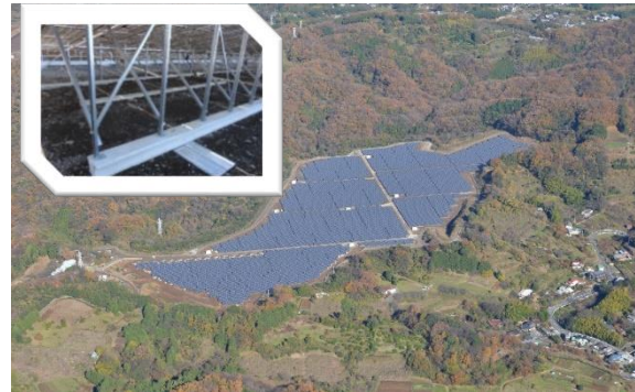
Fig. 7 Ashigara Oi Solar Way H-shaped P.C. laterals and longitudinal piles (source: Japan Asia Group)
