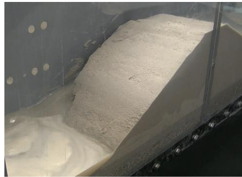
Fig.15 case2 Collapse form
