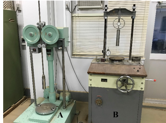
Fig. 3 CBR test apparatus- A) Automated rammer, and B) CBR machine
