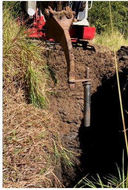
Fig. 1 Insertion of soil sampling tube by the modified adaptor to the excavator's arm
