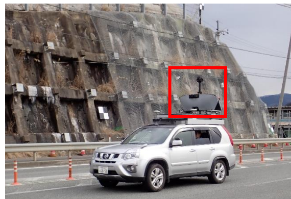
Fig. 2 MMS surveying on the slope (Devices are marked by the red rectangle)
