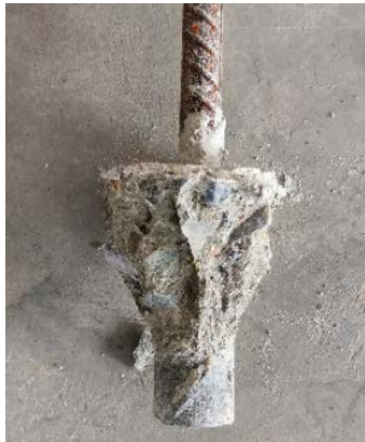
Fig. 12 Concrete conic frustum of cast in place rebar in pull out test.
