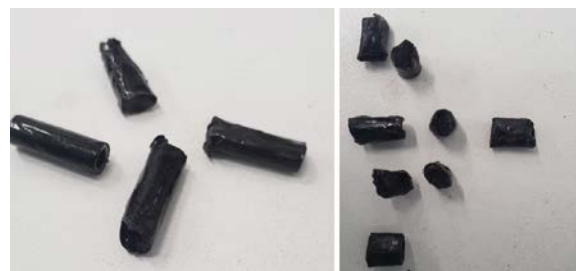
Fig. 7. Sections of Bitumen encapsulated CBs.
