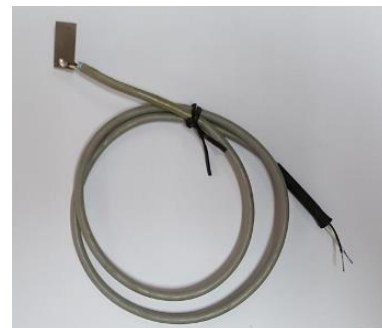
Fig. 5 Connecting the power cable to the bender element.
