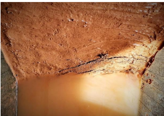
Figure15: Generation of cracks at the toe of the slope.
