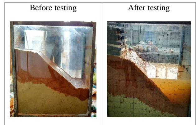
Figure12: Conditions of the 30° slope, before and after the testing. There were no changes after testing in the slope except for the surface erosion created by the artificial rainfall.
