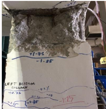
Fig. 13: Spalling of concrete occurred at +1.75%
