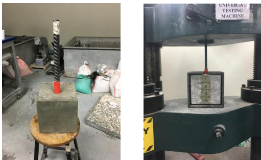
Fig. 1 Concrete cube sample under pull out test
