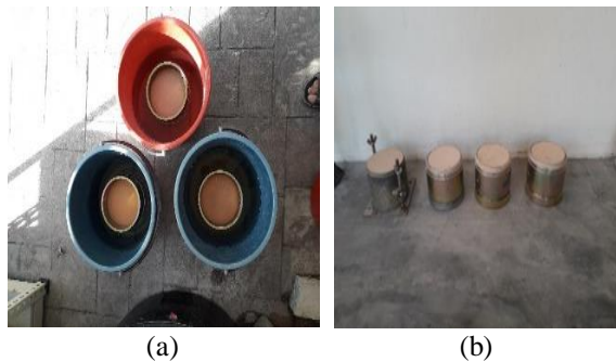
Fig 2: (a) Specimen under water to simulate flood and (b) placed in outdoor area
