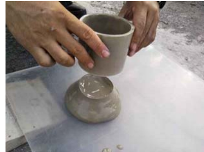
(a) Spread in table flow test ( C.F. = 120 mm)
