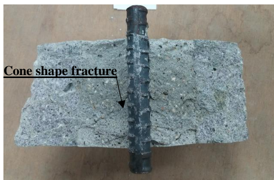
Fig.9 Cone shape fracture ( \ell=65 (mm), d=80 (mm))
