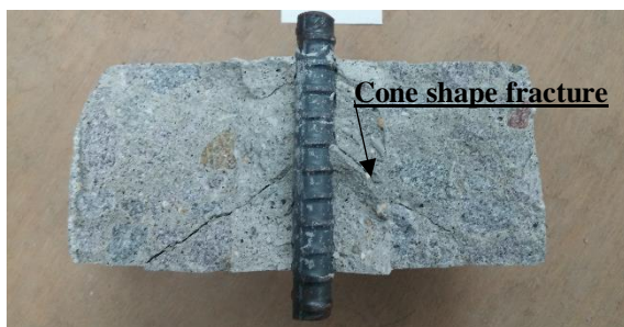
Fig.8 Cone shape fracture ( \ell=65 (mm), d=60 (mm))
