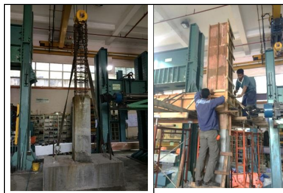
Fig. 6: Construction of corner beam-column joints inside the Heavy Structural Laboratory.
