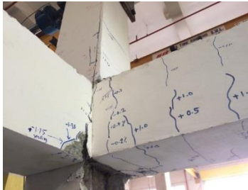
Fig. 12: Vertical and horizontal cracks were occurred on the beam starting from +0.5% drift
