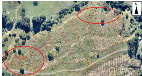
Fig. 3 RTK-GPS movement map of the monitoring site highlighting the two circled areas with significant recorded movement
