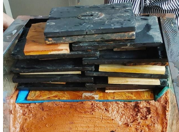
Figure 6: Applied 120 kg surcharge load. The loads were balanced by placing them on wooden pieces, to keep them steadier.
