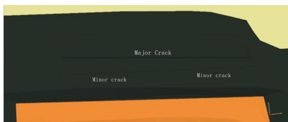
Fig.8 Aerial view of cracks on the north batter surface
