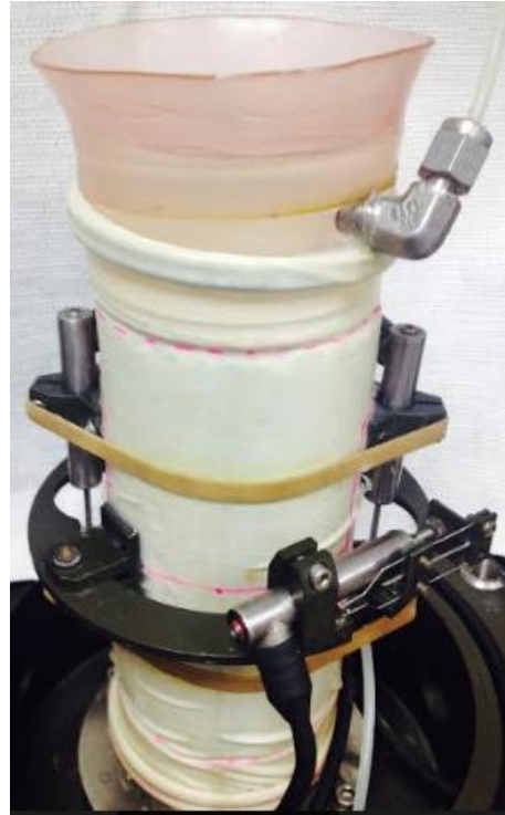
Fig. 2 Local sensors installed on the soil specimen.
