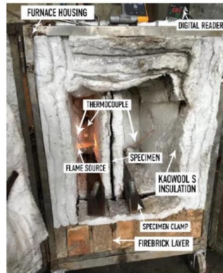
Figure 1. Small-scale furnace for fire testing [16]
