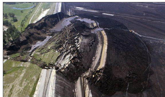
Fig. 1 Yallourn batter sliding on 14th November 2007 [5]
