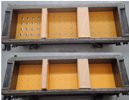
Fig. 1 Steel mold with wood plates having various sizes of round screws
