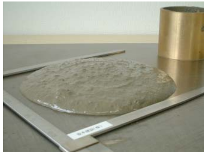
(a) Spread in table flow test ( C.F. = 200 mm)
