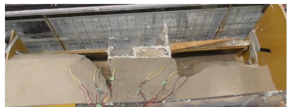
Fig. 13 Scour-like erosion and flow at the upstream side (Case 3)
