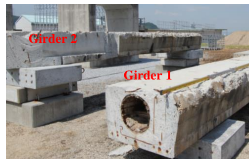
Fig. 5 PC digit removed due to salt damage
