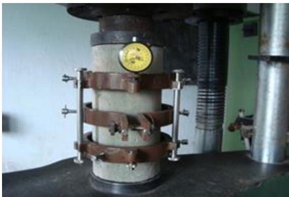
Fig 2: Photo view of set up for modulus of elasticity test
