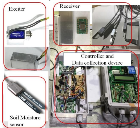
Fig.8 Elastic wave monitoring devices. It can automatically generate elastic wave and measure wave signal.
