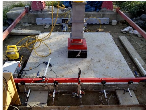
Fig. 11 Positioning of the sensors for experiment with horizontal load.
