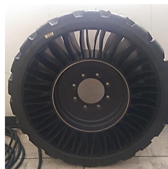
Fig. 1 NPT Tweel 12N16.5 SSL ALL TERRAIN.
