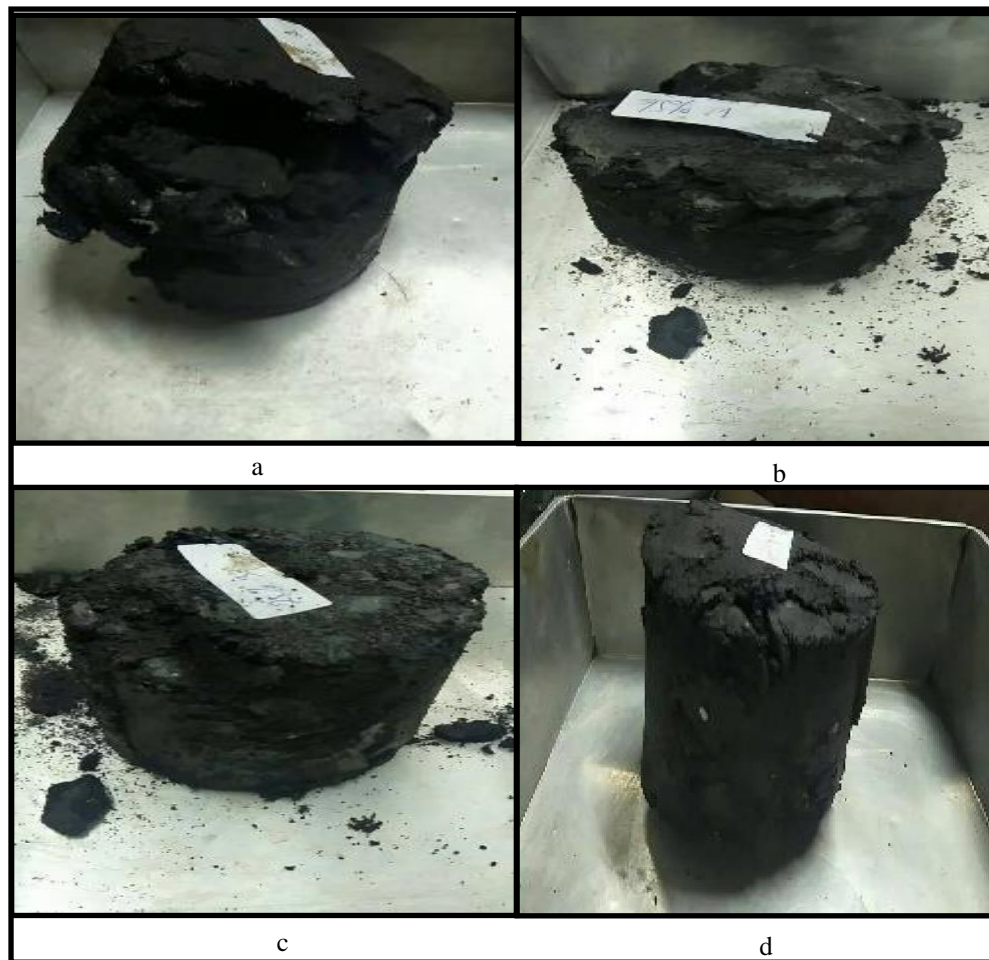
Figure 3 Sample Condition after Marshall Test is Conducted, (a) Sample with 0% tailings (b) Sample with 25% tailings (c) Sample with 50% tailings (d) Sample with 75% tailings
