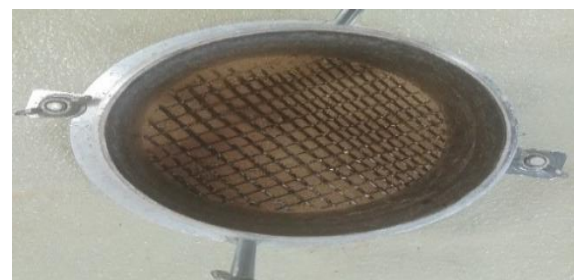
Fig. 5 GGR sample laid or flattened on a surface of a compacted soil layer inside the CBR mold.
