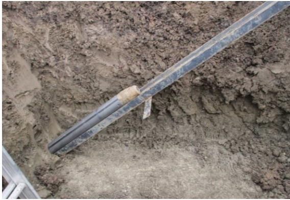
Fig.1 Shelby tube clay foundation sample with inclined orientation
