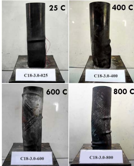
Fig. 4 Failure modes of CFST columns after different elevated temperatures
