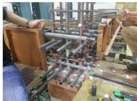
Fig. 5: Installation of fuse-bars at corner joint
