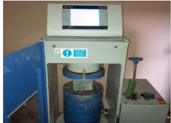
Fig 2 Loaded concrete cube specimen for Compressive strength test
