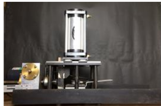
Fig. 5 A vertical loading device
