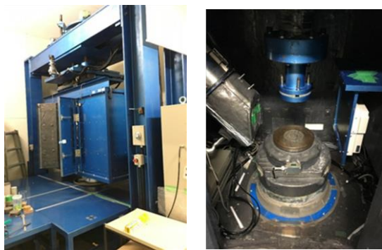
(a) Exterior (b) Interior Figure 2 X-ray CT scanner system
