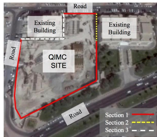
Fig. 3 Division of shoring system along the perimeter
