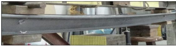
Fig. 6 Lateral-torsional buckling failure
