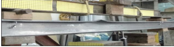
Fig. 5 Distortional buckling failure
