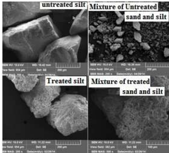
Fig. 8 SEM images of untreated and treated soil grains [11].
