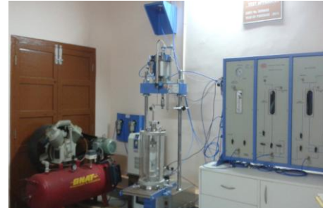
Fig. 2 Photographic overall view of the cyclic triaxial system at CED, NIT Calicut
