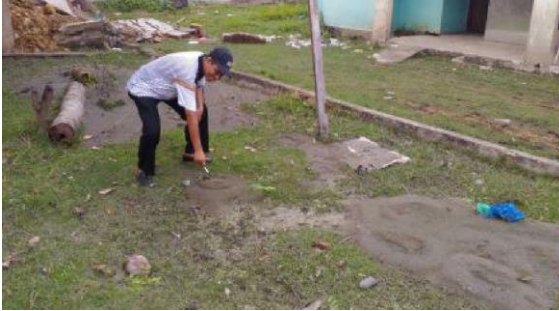
Fig. 3 Sand boil due to Aceh earthquake 2016
