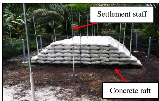
Fig. 2 Setting up of raft for non-uniform loading
