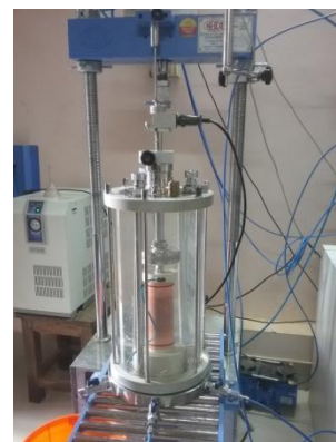
Fig. 4 Soil sample in the triaxial cell
