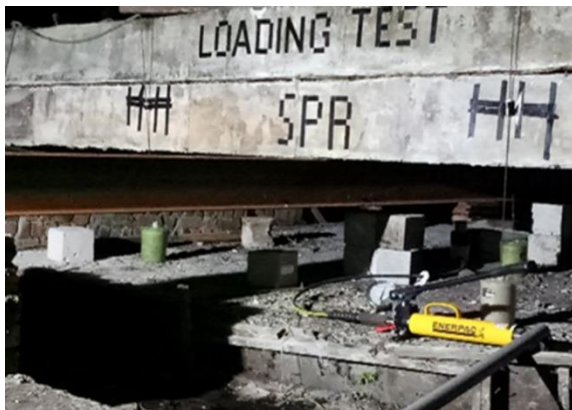
Fig. 5 Hydraulic jack in operation during loading test
