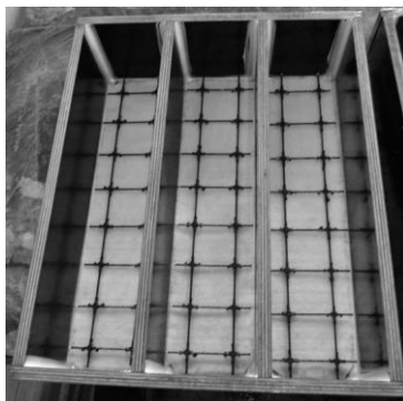
Fig. 4. Basalt mesh on geotextile in the form.
