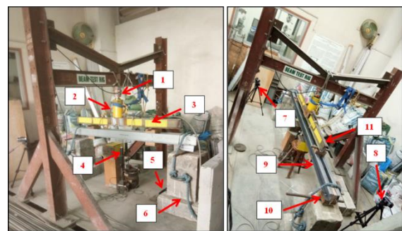
Fig. 3 Actual setup of four-point bend test
