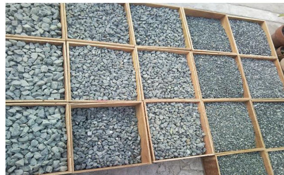
Fig. 1 Crushed coarse aggregates sizes (25mm, 19mm, 12.5mm and 10mm)
