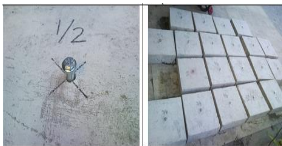
Fig. 2 Installed expansion anchor bolts in concrete bases
