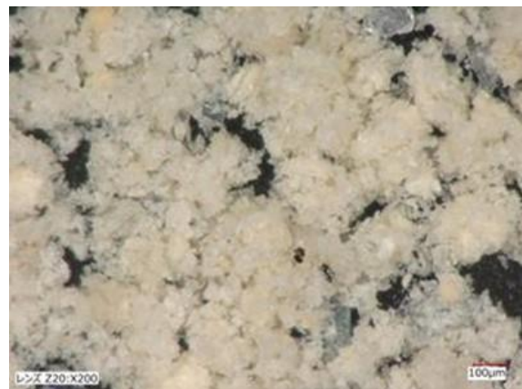
Photo. 6. State after the compression: Pumice
