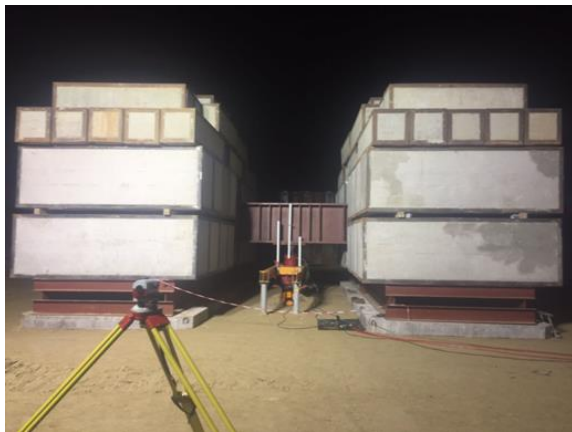
Fig. 4 Testing platform for static compression load test.
