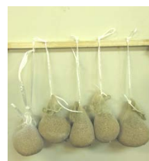
Fig. 2 Zeolites 4A set in experiment tank
