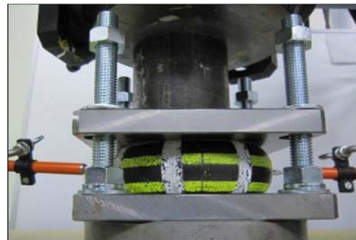
Fig 1. Deformation of rubber (compressive test)
