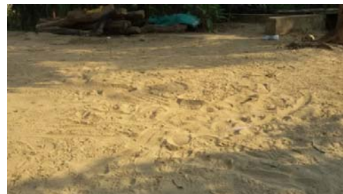
Figure 5 Fine sand ejected through ground cracks.
