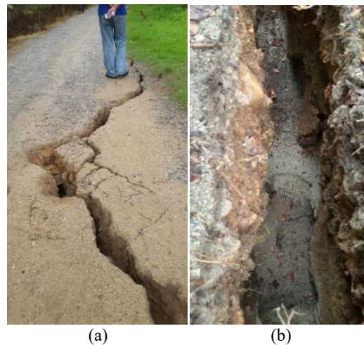
Figure 4 (a) Ground cracking occurred all over the village (this picture was taken at the primary school of the village,) (b) Pure sand appeared at the bottom of the cracks.
