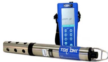
Fig. 1 Portable multi-item water quality meter WQC-24
