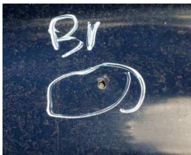
Fig. 1 A defect caused by welding process.
