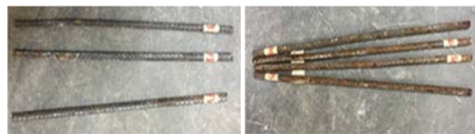
Fig. 7 Steel bar from seawater beam (left), steel bar from freshwater beam (right)
