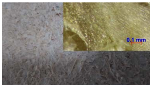
Fig.12 Plubplueng artificial paper : 15 minutes boiled in 4%w/v ashes, 3 hrs. incubated at 100 °C.
