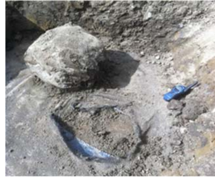
Fig. 2 Liner damage caused by large aggregate.
