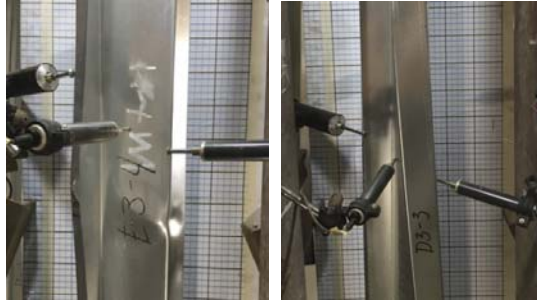
Fig. 4 Failure due to torsional-flexural buckling (right) and distortional buckling (left)
