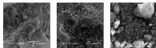
Fig. 2. Microfabric of 100S (5000x, 1000x and 500x Magnification)
