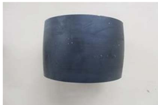
Fig.7 Plastic deformation of specimen
