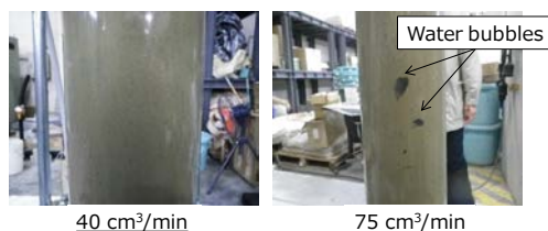
Fig. 10 View of the impervious material after underwater placement
