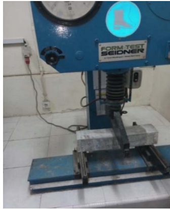
Figure 8. Flexural Test on Beam
