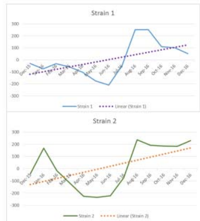
Fig. 11 Strain for Class 1 & 2 vehicles.
