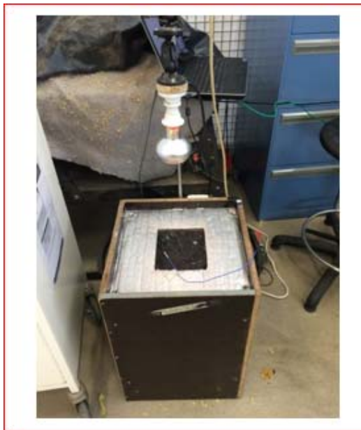
Fig. 10 Heat box and thermal lamp constructed to enable pavement insolation to be varied in a controlled manner (Gray 2014).
