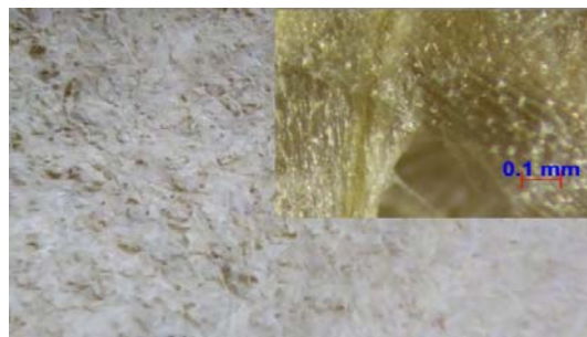
Fig. 10 Plubplueng pulp artificial paper :10 minutes boiled in 4%w/v ashes, 3 hrs. incubated at 100°C
