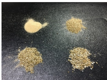
Fig. 4 Toyoura standard sand (upper left), vermiculite of 0.7mm (upper right), 1.0mm (lower left), 2.0mm (lower right)
