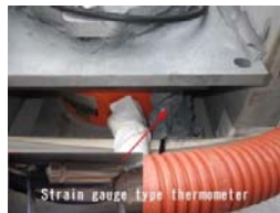
Figure 13 Temperature sensor attached to a load-cell
