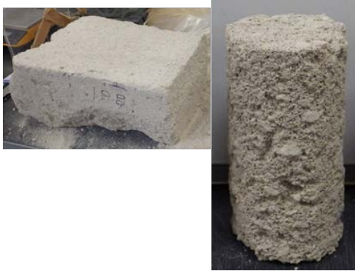
Photo 1 This is a block and a specimen of 24-year-old bubble-mixed solidified soil
