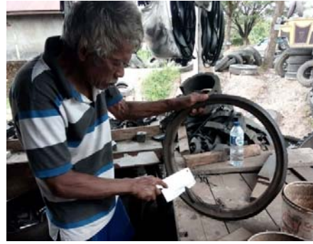
Figure 2. Cutting Process From Waste Tyre to Obtained Steel Fiber Extracted
