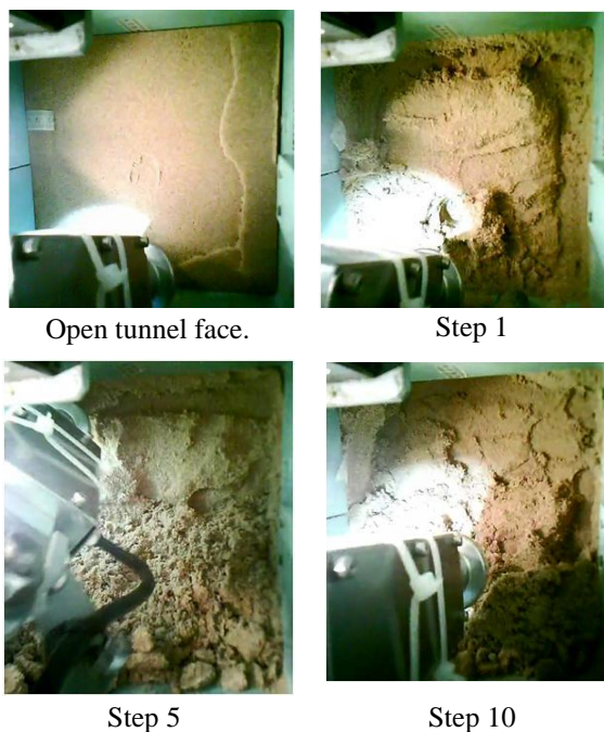
Fig. 8 Tunnel face changes by miniature camera.
