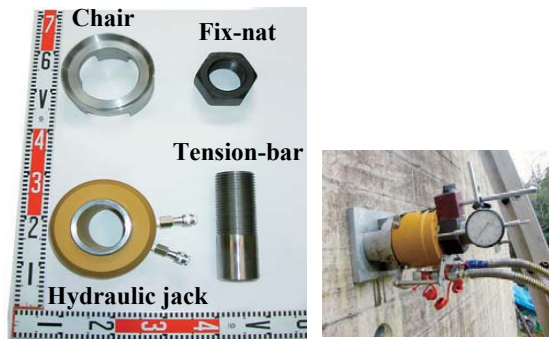
Figure 2 Components and installation of the SAAM jack.
