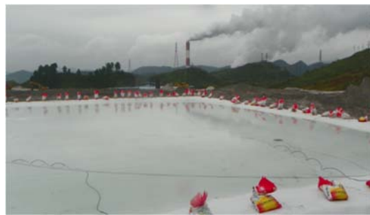
Fig. 13 Lined test pad flooded with acid water.
