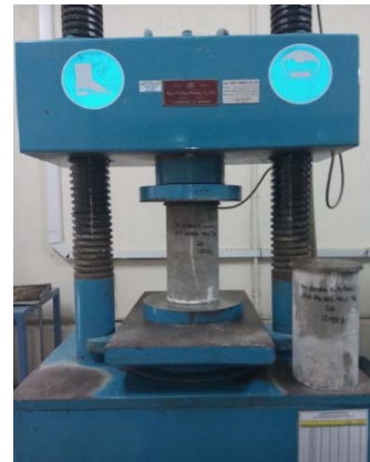
Figure 6. Compressive Test on Cylindrical
