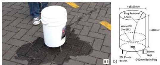
Fig. 6. Stormwater infiltration field test (SWIFT) Infiltrimeter used in this study. (a) SWIFT in use; (b) SWIFT dimensions [44].
