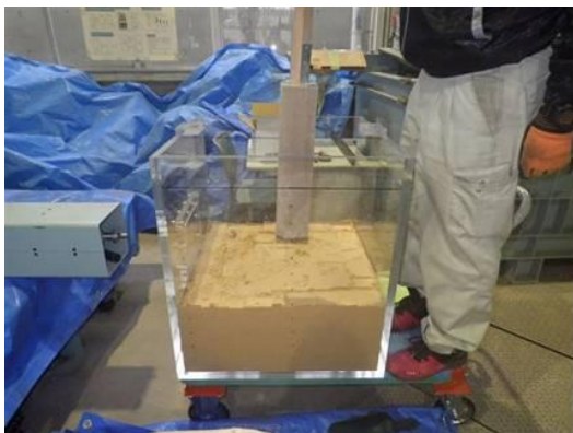
Fig. 6 Compacting sand layer in each 50 mm height.
