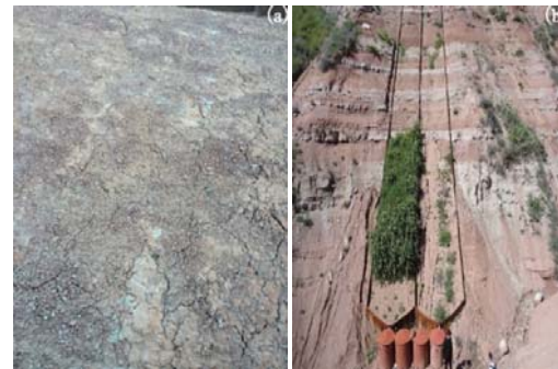
Fig. 3 Comparison of experimental and control area. (a) a few cracks in consolidation and water proof area, (b) comparison with two plots in September, 2014
