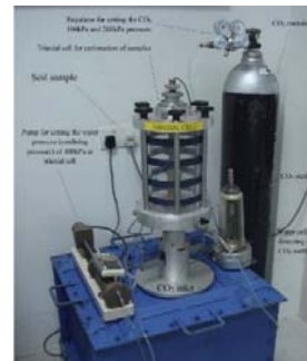
Fig. 7 Cell setup for carbonating olivine treated soil.
