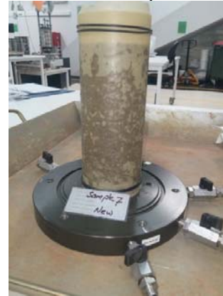
Fig. 4 New specimen confined by membrane
