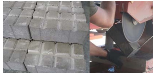
Fig. 7 – Sediment Slots Being Cut into Underside of PICP blocks [28]
