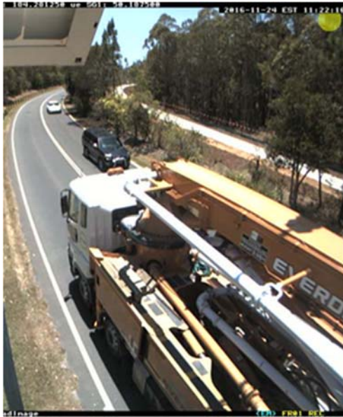
Fig. 10 A concrete pumper has exceeded the 'trigger' strain value.
