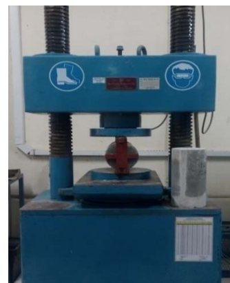
Figure 7. Splitting Tensile Test on Cylindrical
