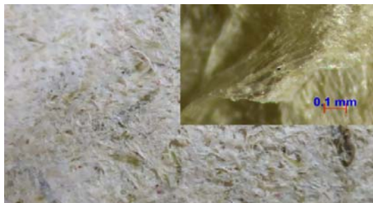
Fig. 9 Plubplueng pulp artificial paper : 10 minutes boiled in 3%w/v KOH, 3 hrs. incubated at 100°C
