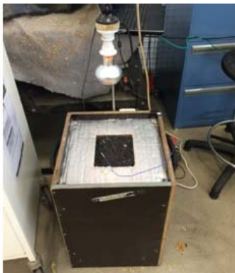
Fig. 10 Heat box and thermal lamp constructed to enable pavement insolation to be varied in a controlled manner (Gray 2014).
