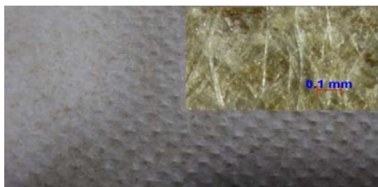
Fig. 7 Puttaraksa artificial paper : 15 minutes boiled in 4%w/v KOH, 3 hrs. incubated at 100 °C.
