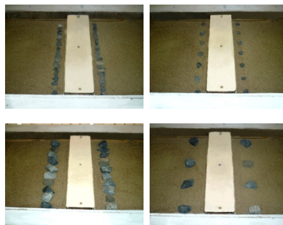
Fig. 2 Gravel chippings arrangement while experimenting with effective parameters of perimeter plate outline reinforcement.
