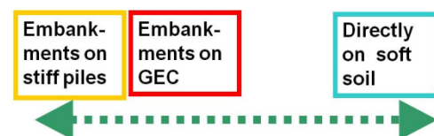
Fig. 10 Position of the GEC System between two extrema: embankments on rigid elements and embankments without any support.
