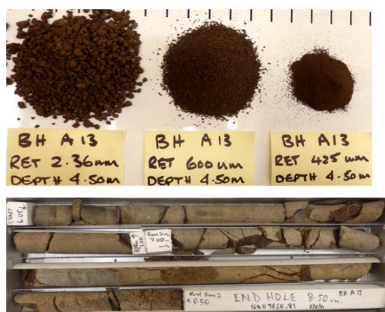
Fig. 3 Moderately weathered basalt obtained via TC Bit and NMLC core drilling techniques
