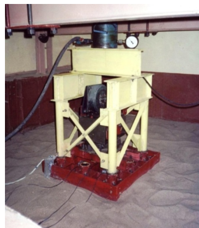
Fig. 6 Experimental studies perimeter reinforced base of the square plate 5,000 cm 2 in area in the big soil tray on small packed sand (the loading device includes directional vibrator and allows transfer of vertical or horizontal dynamic loads to the plate in addition to static loads – this article does not examine the dynamic tests results).
