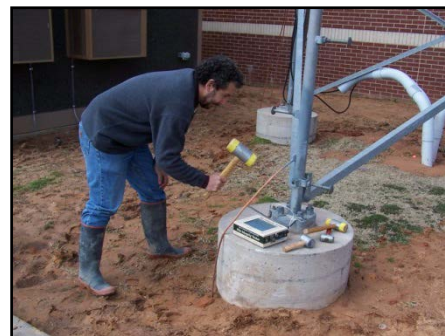
Fig. 1 Concrete pile subjected to low strain integrity test [7].
