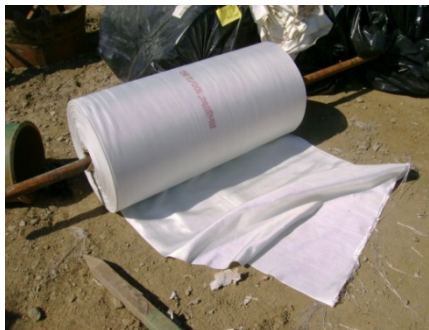
Fig. 4 Typical woven seamless encasement as delivered to the site before installation.
