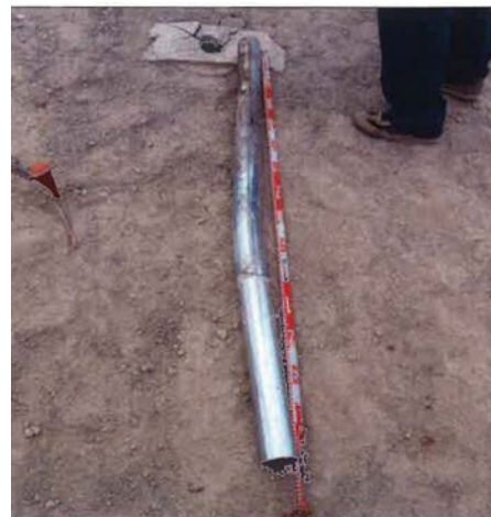
Fig.13 Bending failure of steel pipe after lateral test
