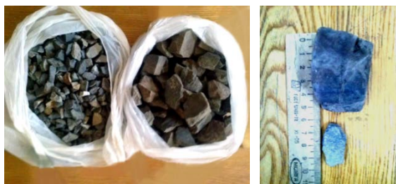
Fig. 1 Gravel chippings of different size, shaping solid incompressible inclusions in experiments on outline reinforcing in a small ground tray.
