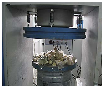
Fig. 10 Bursting formation under fast loading rate
