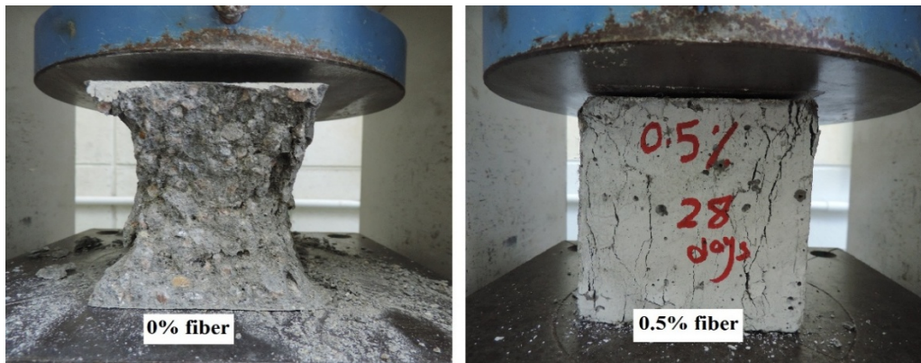
Fig. 2 Failure mode of concrete cube under compressive load.
