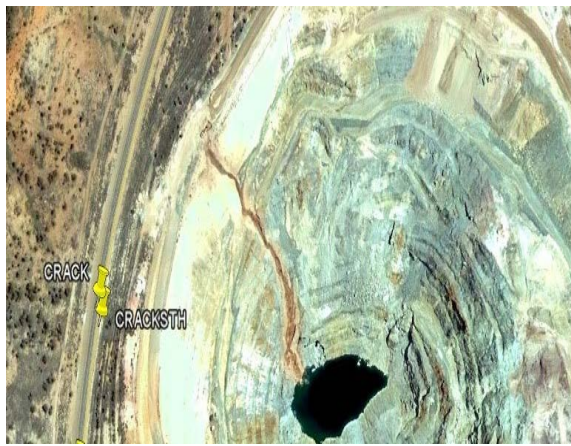
Fig. 1 Location of cracking on the roadway in relation to the mine.
