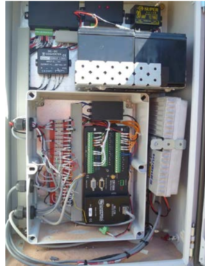
Fig. 6 Telemetry system showing data logger, modem, power management and batteries.
