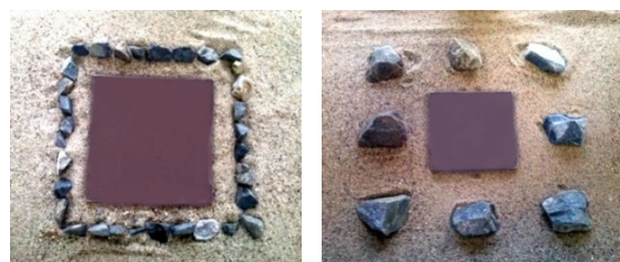
Fig. 3 Gravel chippings arrangement while experimenting with effective parameters of square plate outline reinforcement.
