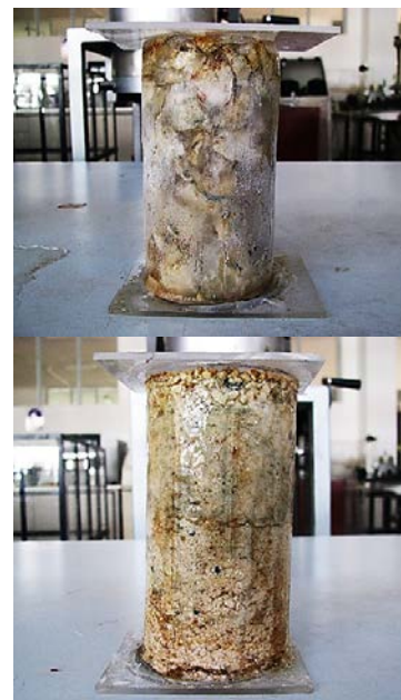
Fig. 9 Failure mode and observed cracks on the samples a. gravel sample, b. sandy sample
