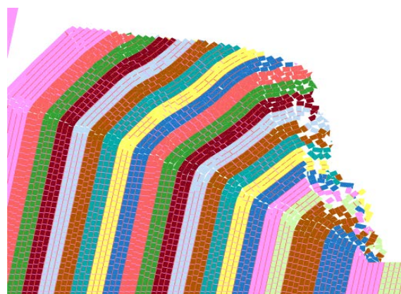
Fig. 7 Rock falls at 60^\circ slope face angle and 0.017 bed-height ratio
