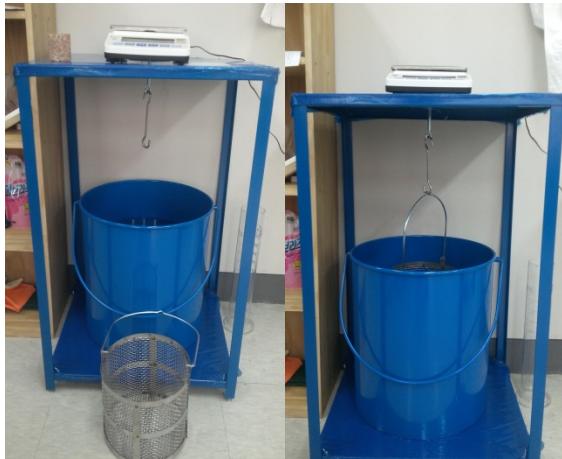
Fig. 2 Equipment to measure the submerged weight
