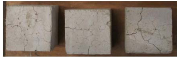
Fig. 5. OPC after elevated temperatures of 1000 °C for 3 hours and cooling in open area for 2 hours.
