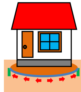
Fig. 1 Image of tensile force around geosynthetics
