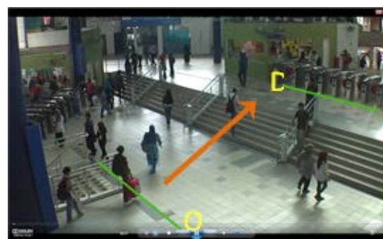
Figure 7: Movement direction of passenger from escalator/elevator (point O) to ticket gates (point D).
