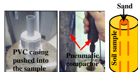
Fig. 2 Preparation of composite specimen
