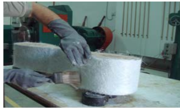
(c) '8' shape glass fiber geomaterial preparation
