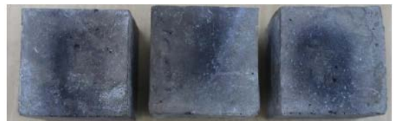
Fig. 8. OPC-Kaolin-bentonite after exposed to elevated temperatures of 500 °C for 3 hours and cooling in water immediately.
