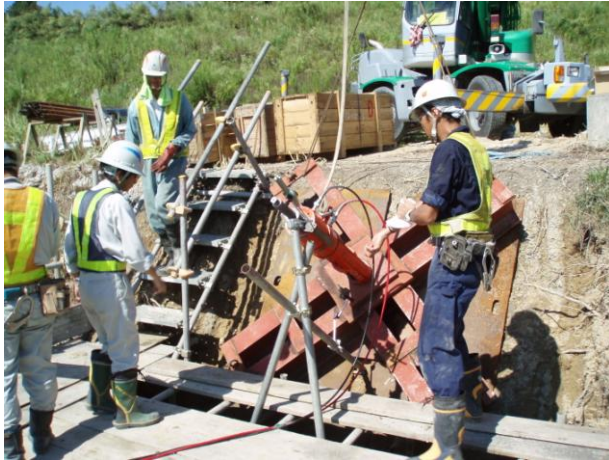
Photo 6 Pullout Test Revealed \tau = 0.5 \text{ MN/m}^2 for a Project in the Makinohara Region
