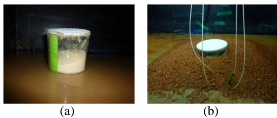
Fig. 18 Situation of the Manhole (1 st earthquake): (a) Manhole Without Countermeasure, (b) Manhole With Countermeasure
