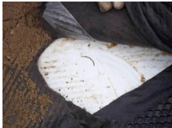
Fig. 8 Photo of defect found during covered ELI survey
