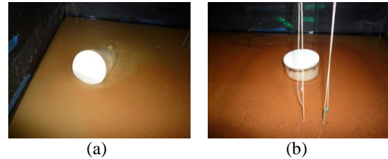
Fig. 19 Situation of the Manhole (2 nd earthquake): (a) Manhole Without Countermeasure, (b) Manhole With Countermeasure
