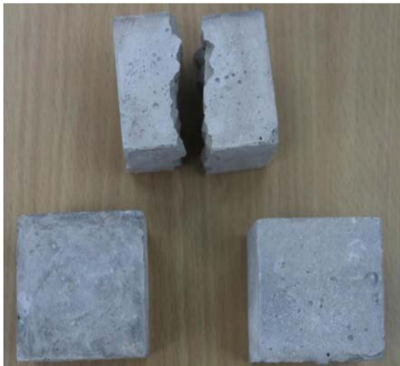
Fig 4. OPC-Kaolin-bentonite after exposed to elevated temperatures of 500 °C for 3 hours and cooling in open area for 2 hours.
