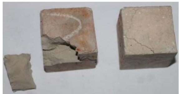
Fig. 7. OPC after exposed to elevated temperatures of 500 °C for 3 hours and cooling in open area for 2 days.
