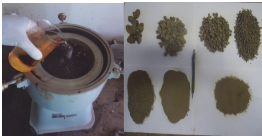
Figure 11 Extraction of asphalt binder and aggregate recovery.
