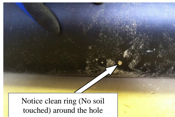
Fig. 3 Hole over imperfection in subgrade
