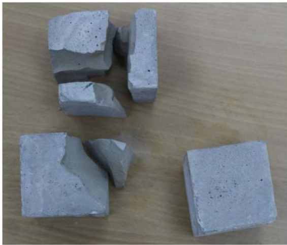
Fig. 3. OPC after exposed to elevated temperatures of 500 °C for 3 hours and cooling in open area for 2 hours.
