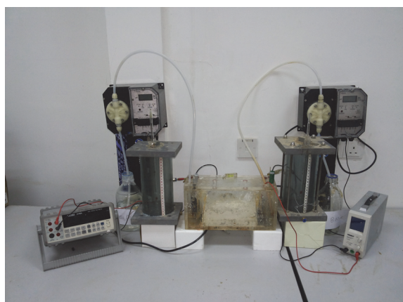
Fig.1. a) Schematic diagram of Electro-biogrouting setup
