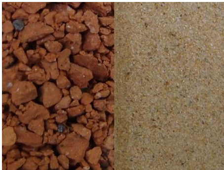
Fig. 2 Shape of the particle of material (Left side: crashed tile, Right side: Toyoura sand)
