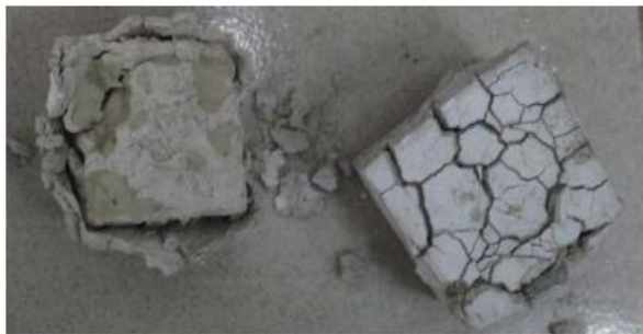
Fig. 9. OPC-Kaolin-bentonite after exposed to elevated temperatures of 1000 °C for 3 hours and cooling in water after 2 hours.
