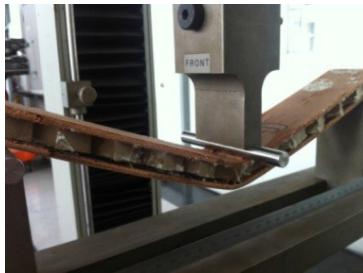
Fig. 14 Load at peak of PU specimen testing.
