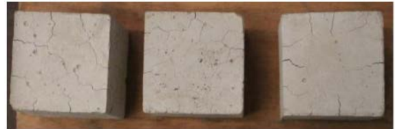
Fig. 6. OPC-Kaolin-bentonite mixture after exposed to elevated temperatures of 1000 °C for 3 hours and cooling in open area for 2 hours.
