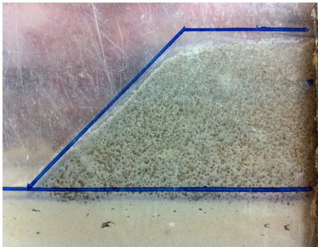
Fig. 11. Deformation behavior of model III (unreinforced embankment on soft foundation)
