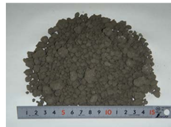
Figure 1 Cement-treated granular soils (CTGS) prepared for centrifuge model tests
