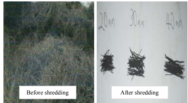
Fig. 1: Recycled steel fibre before and after shredding.
