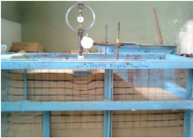
Fig. 9 Deformed shape profile of soil under the footing at failure.
