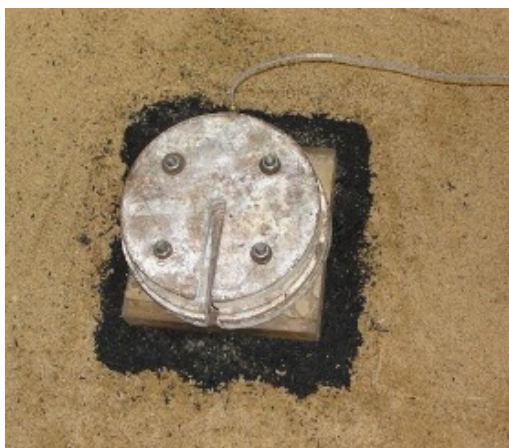
Figure 8. Model footing resting on 50% shredded rubber and sand mixture.
