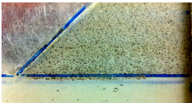
Fig. 17. Deformation behavior of model V (reinforced embankment on soft foundation)
