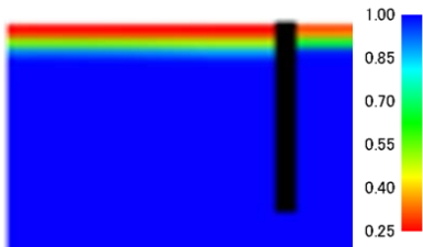
Fig.10 Distribution of degree of saturation around the pine's root system (CASE-2)
