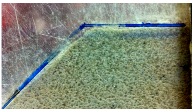
Fig. 16. Deformation behavior of model V (reinforced embankment on soft foundation)
