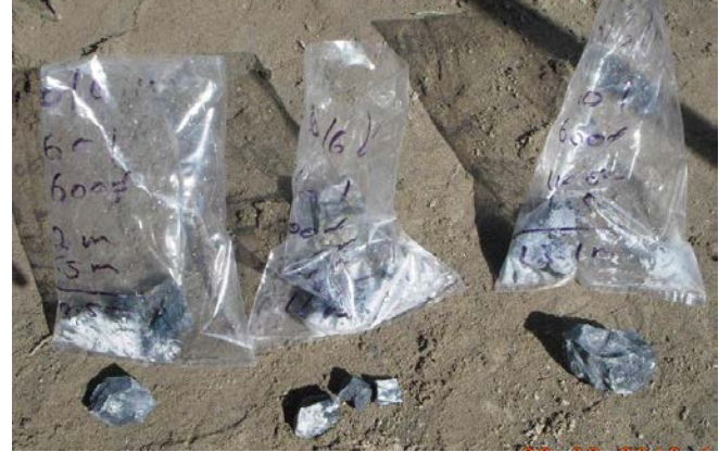
Fig. 4. Excavation spoils collected from various boring depths.
