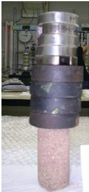
Fig. 2. Sand column treated by biocement
