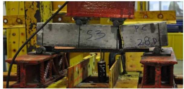
Fig. 6: Failure mode of plain concrete beam in flexure.
