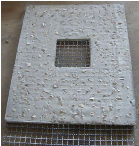
Fig. 3 Completed composite reinforcement containing ASH
