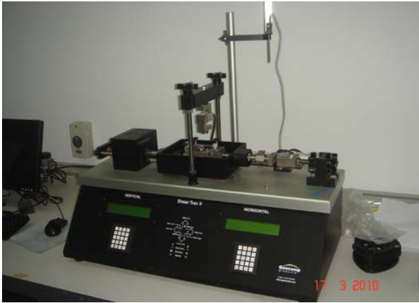
Figure 1 ShearTrac II direct shear system
