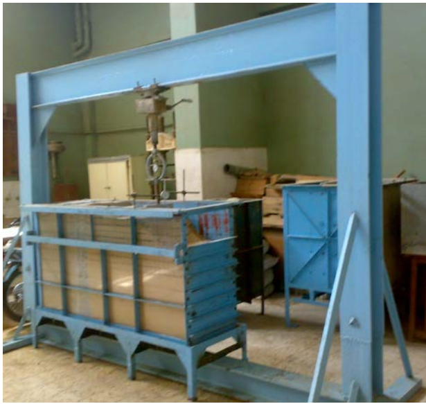
Fig. 4 Sand container mounted under loading frame
