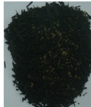
Figure 7. Magnified view of 50:50 sand and shredded rubber tire mixture.
