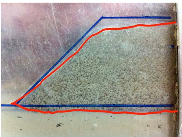
Fig. 12. Deformation behavior of model III (unreinforced embankment on soft foundation)
