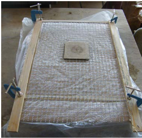
Fig. 2 Mold for cast composite reinforcement
