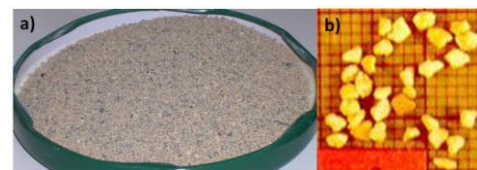
Fig. 2.2 Tested materials. a) debris flow material; b) natural sand.
