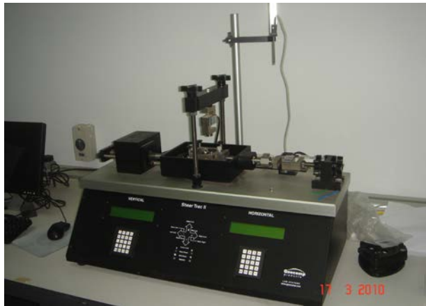
Figure 1 ShearTrac II direct shear system
