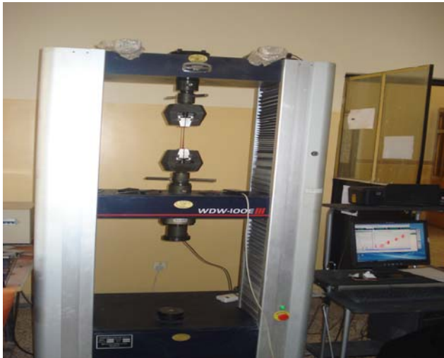
Figure 3: Computer controlled electronic universal testing machine
