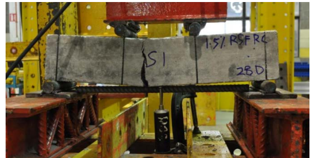
Fig. 7: Failure mode of RSFRC beam in flexure.
