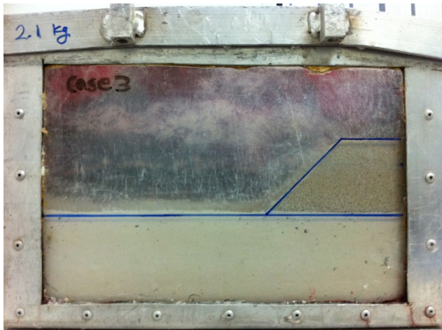
Fig. 7. Embankment on soft kaolin foundation
