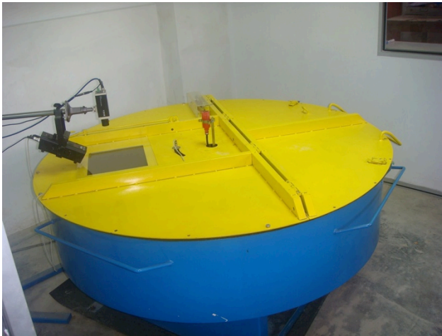
Fig. 1. Overall view of small geotechnical centrifuge apparatus.
