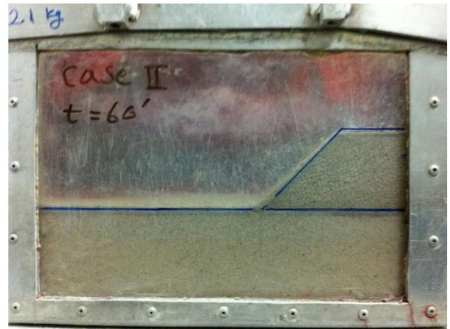
Fig. 8. Deformation behavior of model II (unreinforced embankment on stiff foundation)
