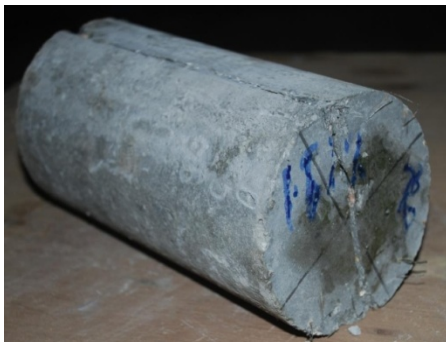
Fig. 5: Concrete cylinder after splitting tensile test.
