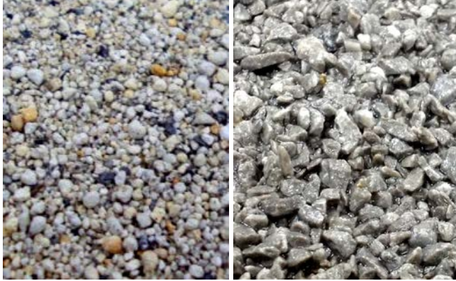
Figure 3 (left) Sample 1 (spoils of metagraywacke); (right) Sample 2 (spoils of sandstone) used for direct shear tests
