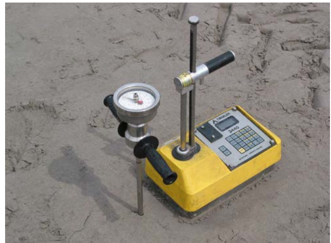
Fig. 9. Troxler gauge and hand CPT equipment during testing tailings [6].
