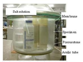
Fig. 2. Applied soil suction .in the glass desiccator.
