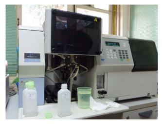
Fig.6 Atomic Adsorption Spectrometer (AAS)
