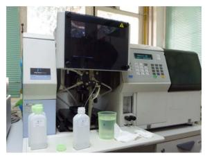
Fig.8 Atomic Adsorption Spectrometer (AAS)
