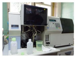
Fig.4 Atomic Adsorption Spectrometer (AAS)
