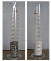
(a) Gravel (left) and the crushed shell particles (right) poured and lightly compacted in the glass cylinder. A solid line shows the height of both the lower cylindrical volumes.
