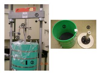
**Figure 2.** Test setup for model pile loading test: ① Adjustable height loading frame ② Test tank ③ LVDT ④ Load cell ⑤ Model pile, ⑥ Compaction base plate.
