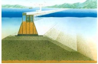
Figure 21: An illustration of cross section of Kamaishi port gigantic breakwater [3].
