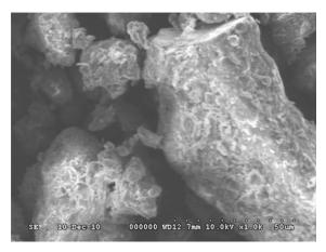
Fig.2 SEM photograph of SM-Soil
