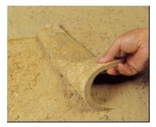
Fig. 4 Appearance of the sand-fixing layer with W-OH
