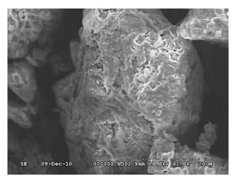
Fig.1 SEM photograph of CL-Soil
