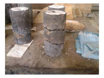
Figure 3.5 Example of typical shear banding and failure characteristics.
