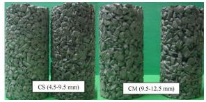
Fig.1 Porous geopolymer concrete specimens
