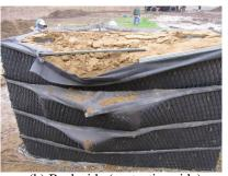
(b) Back side (protecting side) Fig. 20. Piled Geo-wall-1 (PGW-1)
