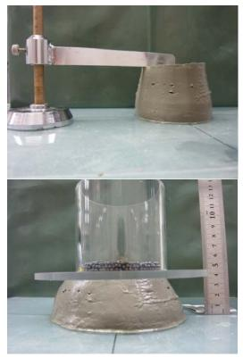
Fig. 9 The conventional slump test and the enhanced test with a burden applied using a specially fabricated cup and small lead balls
