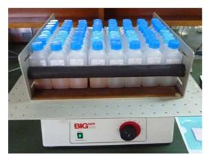
Fig.7 Shaking the mixture of soil and heavy metal solutions
