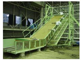
Fig.2 Flume and model slope
