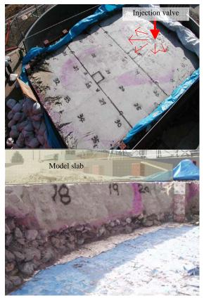
Fig. 6 Surface and section of solidified hydraulic plastic grout after test injection
