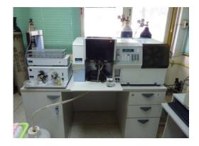
Figure 4. Atomic Absorption Spectrophotometer (AAS).
